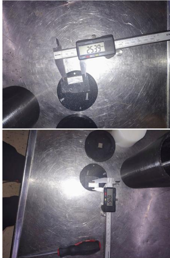
Figure 8b. Sample holder and positioning of indium foil.
