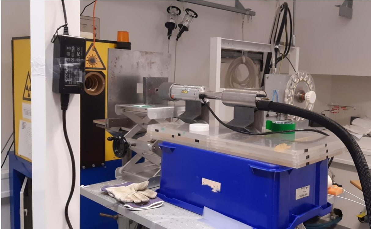
Figure 3: Measurement setup at DSA. The beam from the irradiator was collimated with two additional collimators (tungsten KAP collimator and a lead block with 1 cm hole diameter) before the spectrometer. The fluence entering the detector was reduced further with a 2 mm diameter collimator disk in front of the detector.
