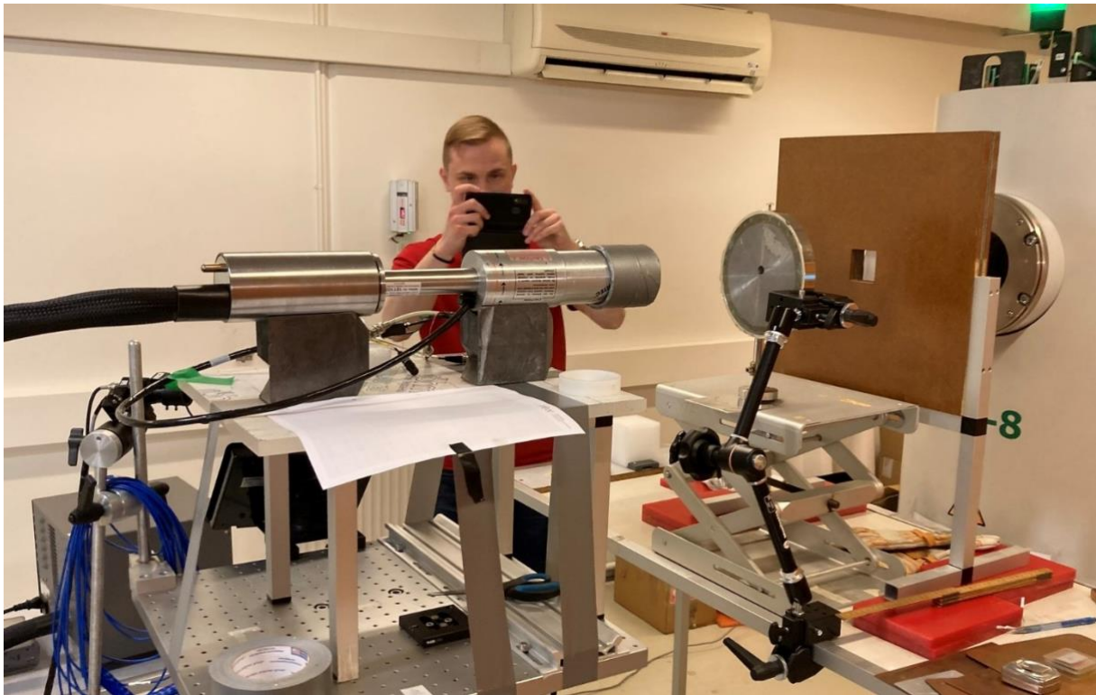
Figure 2: Measurement setup at SIS. The beam from the irradiator was collimated with two additional collimators, a lead KAP collimator and a lead collimator from STUK with 1.4 cm hole diameter, before the spectrometer. The fluence entering the detector was reduced further with a 2 mm diameter collimator disk in front of the detector.
