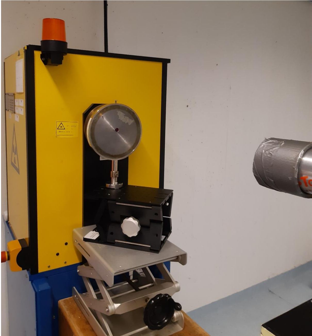
Figure 1: Measurement setup at SSM. The spectrometer lead shielding is visible on the right. The beam from the irradiator was collimated with a 1.4 cm hole diameter collimator from STUK. The purpose of the additional collimator was to reduce the beam size to smaller than the lead shielding around the spectrometer. The fluence entering the detector was reduced further with a 2 mm diameter collimator disk in front of the detector.
