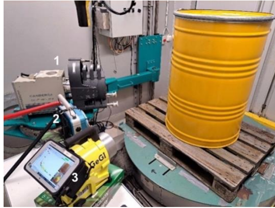
Figure 8: Measurement setup at Svafo, with the HPGe gamma spectrometer (1), H420 gamma camera (2) and GeGI gamma camera (3) observing a 280 liter waste drum.
