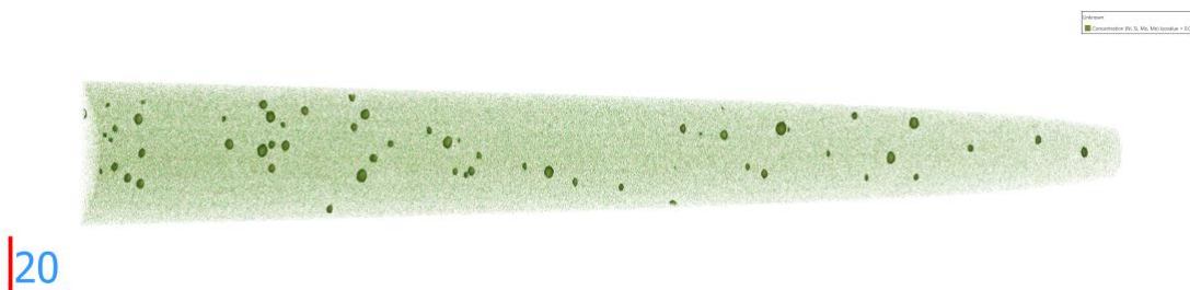
Figure 1. A large APT dataset from the irradiated Barsebäck weld showing clusters.
