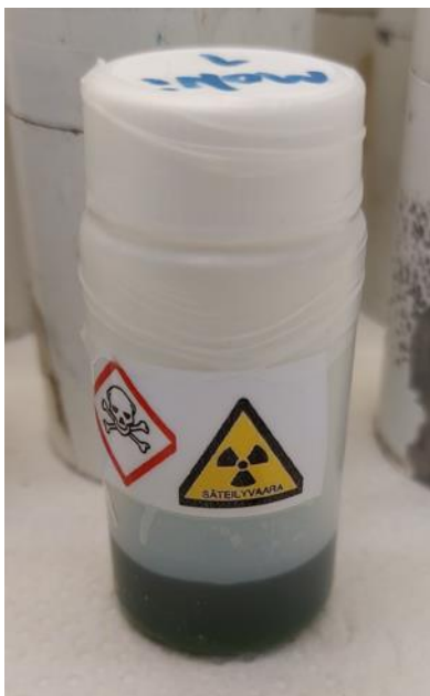
Figure 2. Example of an acid digested sample.
