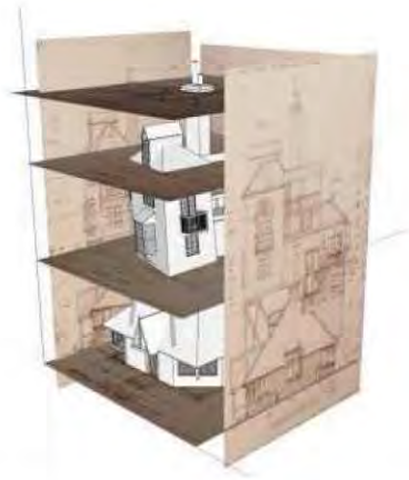
Blueprints/drawings/photos can be used as background to build the 3D model on
