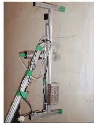
Single axis vertical scanning frame in use at Chapelcross Pond 1.
