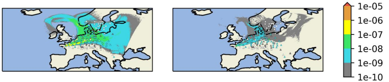
Figure 18 Accumulated depositon of PMCH [ \text{g h/ m}^3 ] of the forward run (left) and the source term from the inversion using all observations equally weighted (right). Triangles show the accumulated concentrations with white triangles marking no detections during the experiment.
