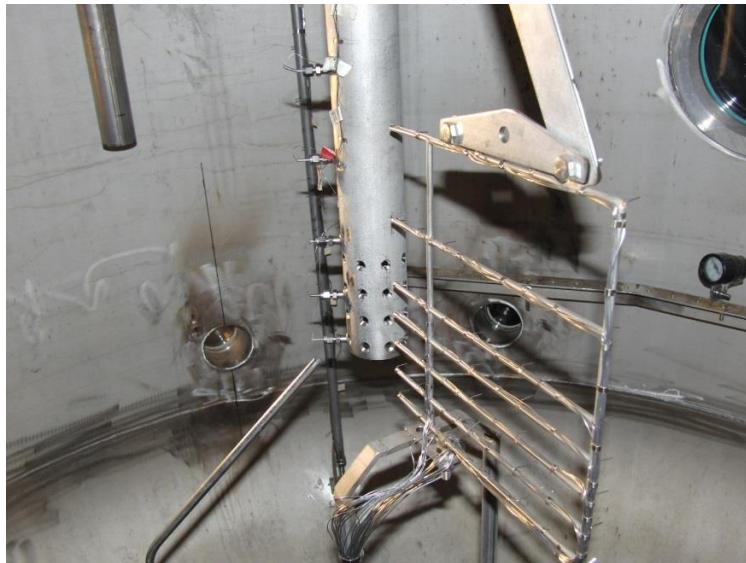
Figure 2-2. Sparger of the PPOOLEX test facility (Laine et al., 2015).
