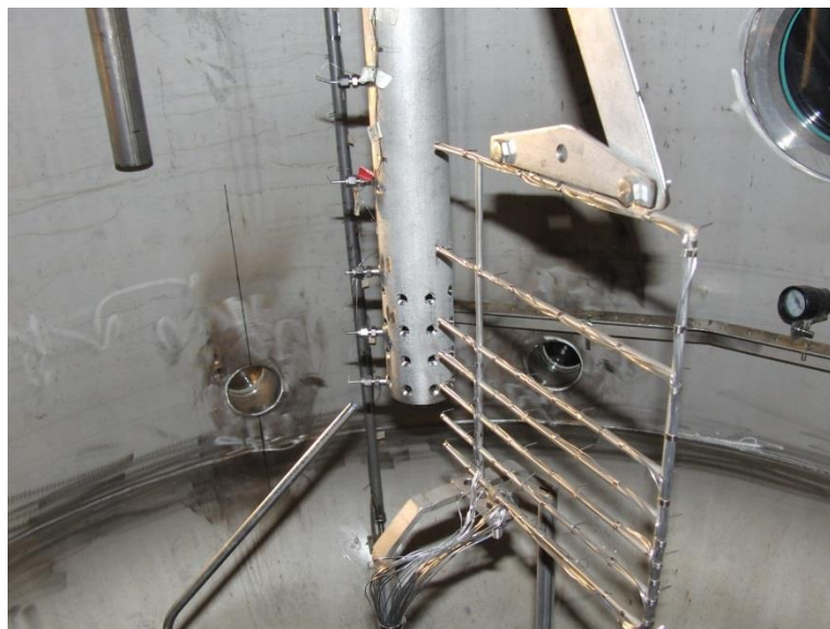
Figure 2. Sparger pipe in the pressure suppression pool of the PPOOLEX test facility at the LUT University (Laine et al., 2015).
