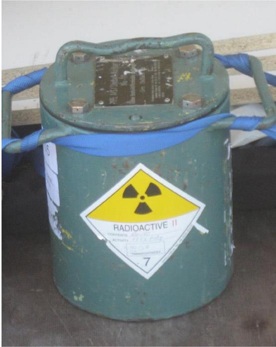
Fig 3.3. The shielded source container with the Co-60 sources used in the shielding experiment.
