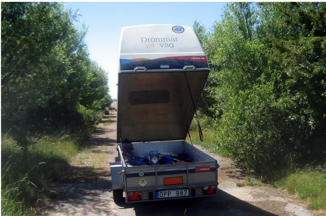
Fig 3.5 The shielded Co-60 source in the trailer for easy movement to different distances from the main road where the vehicles with the mobile spectrometers were parked. The source in the trailer was initially placed 30 m from the main road (2018-06-07 14:00 - 14:20) and then moved to 20 m distance in order to increase the detection probability (14:20 - 14:30).
