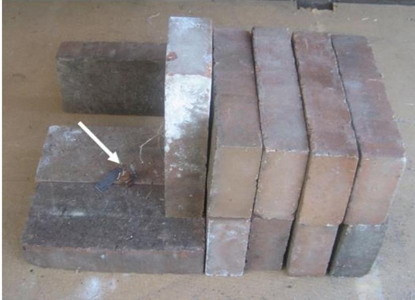
Fig 3.1 Non-collimated source geometry. Point sources of Cs-137 and Co-60 (location indicated by the arrow), were used in this shielding geometry, with 1 - 5 clay bricks and 1 - 7 wooden blocks, in this picture with 5 clay bricks (500 mm) as a shield between the source and the detector. The detector is placed at various distances 1 - 20 m to the right of the shield, depending on the source activity.
