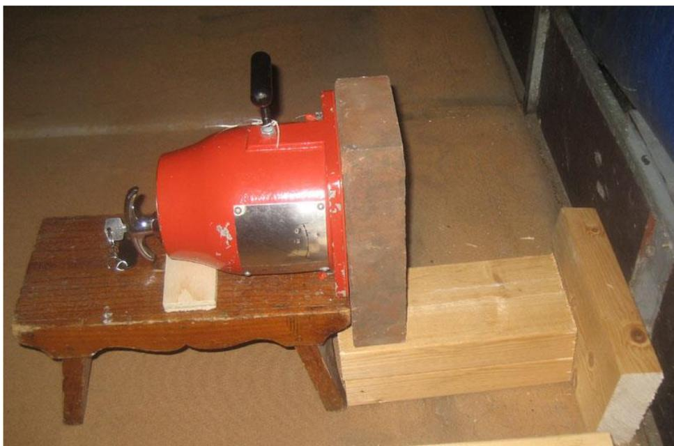
Fig 3.8 Collimated source geometry. Clay bricks (1 - 5 bricks, 50 - 250 mm) were used as shielding material in front of the collimated Cs-137 source, in this picture with one clay brick supported by wood blocks underneath.
