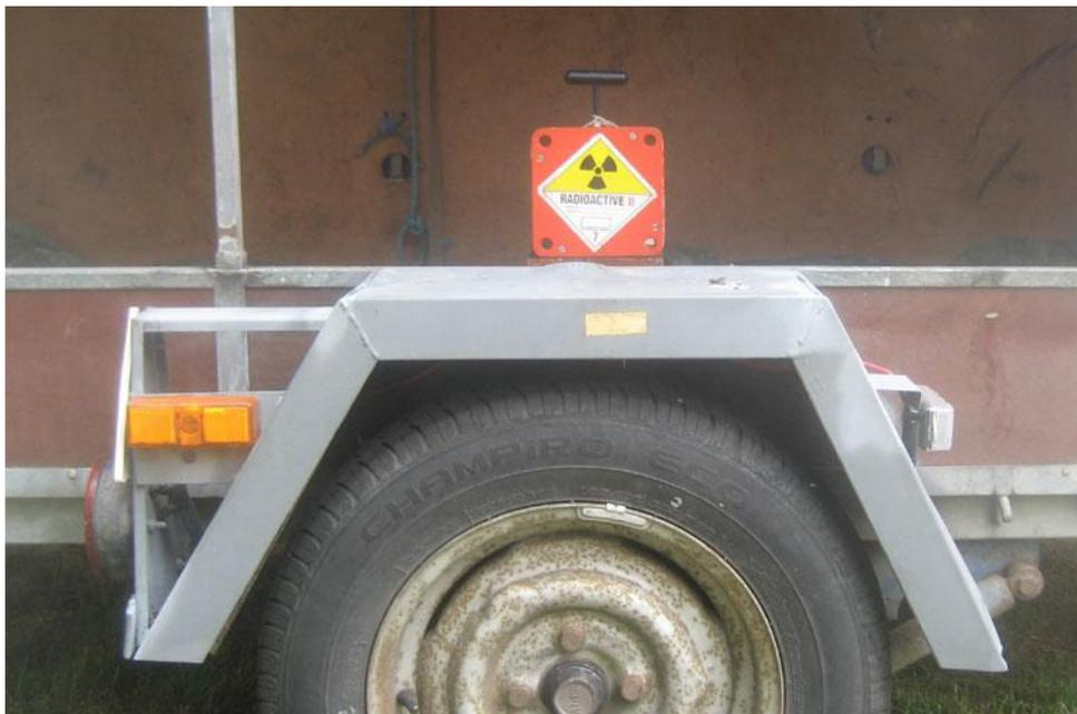
Fig 3.7 Collimated level guard with a 520 MBq Cs-137 source placed in radiation position as seen from the detector location. The distance between the source and the detector was 16.7 m. The opening angle of the collimator, seen from the source towards the detector, was in the horizontal direction 12 degrees and in the vertical direction 18 degrees.
