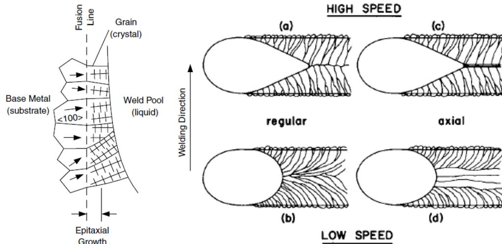
**Figure 2.6.** On the left: Epitaxial growth near the fusion line and weld pool. On the right: Effect of travel speed on the weld pool shape and the columnar grain growth. Axial grains may initiate in the middle of the fusion zone and the speed of the weld pool affects the width of the region of the axial grains. [10]
