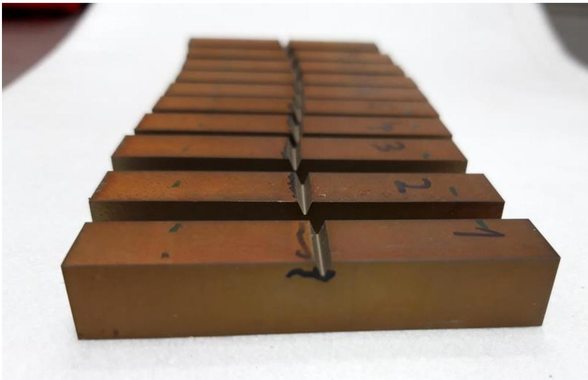
Figure 6. Impact specimens fabricated from trepan 2.
