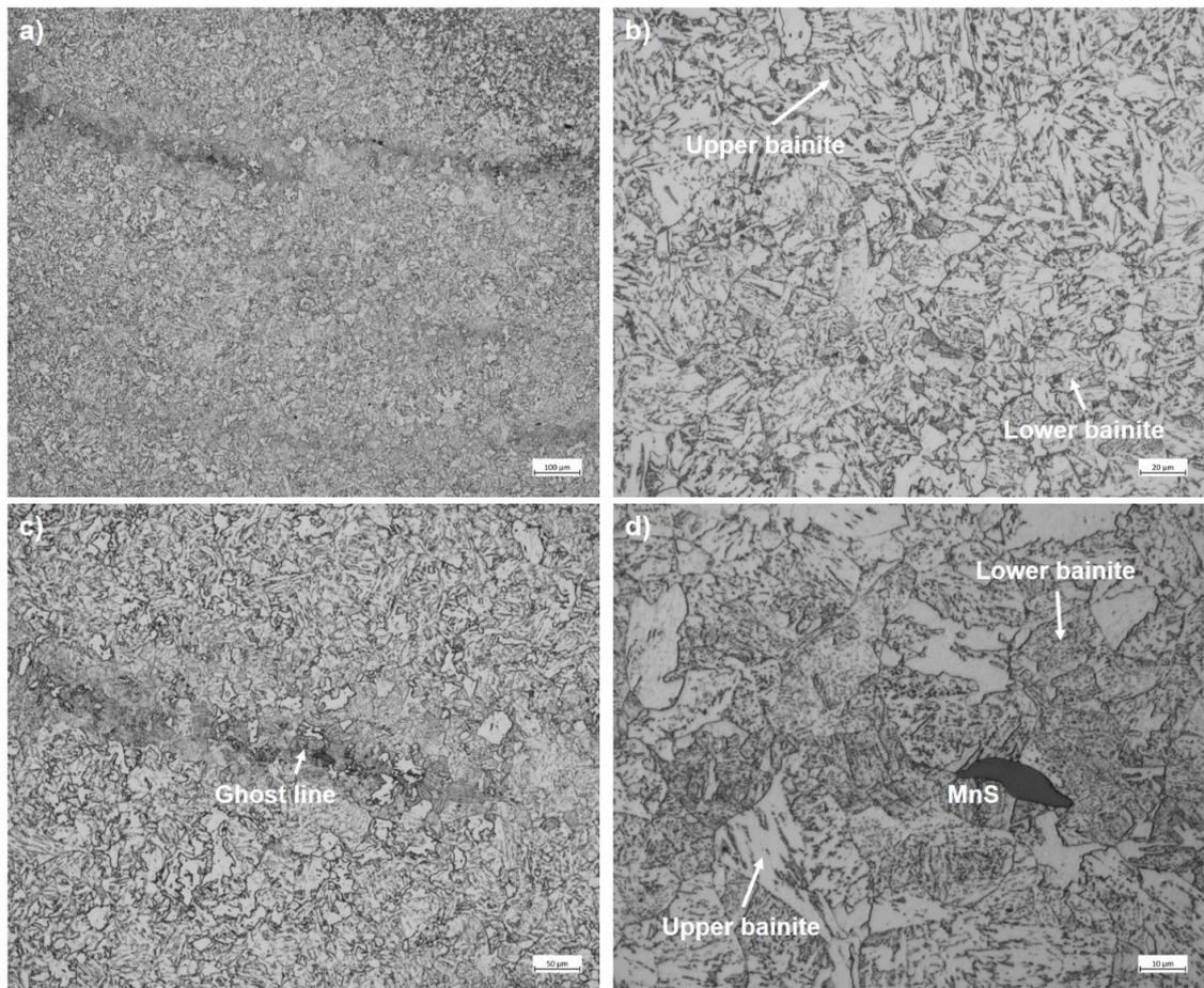
**Figure 5.15.** Images a) and b) show the plate base material on the outer wall side with a MMA weld and typical bainitic microstructure. Images c) and d) show the ghost line microstructure and the manganese sulphide particle.
