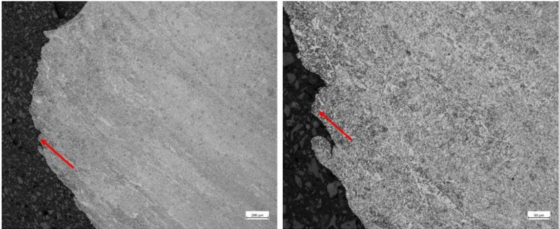
**Figure 5.32.** Microstructure of the cross-section specimen CVN 2B5. The arrows point to the approximate location of the primary initiation site on the fracture surface.
