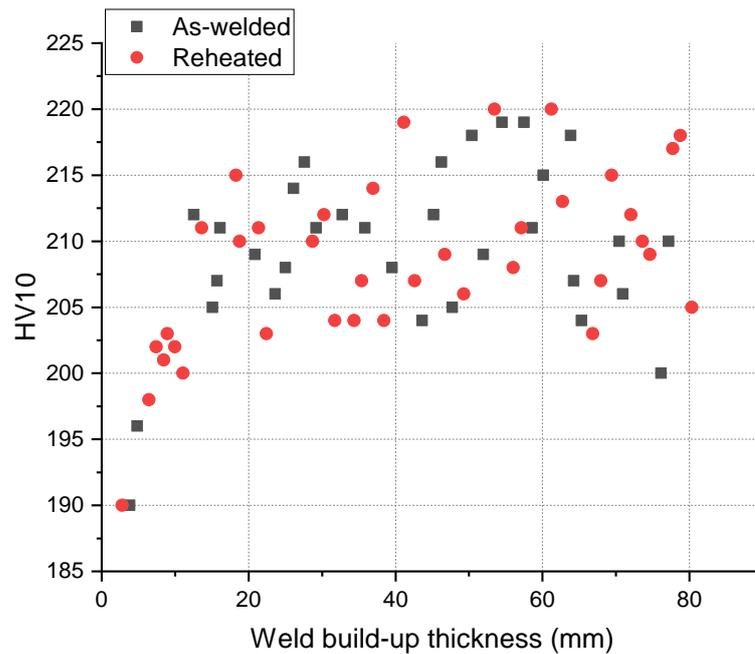
**Figure 5.2.** HV10 results through the wall thickness in the cross-section investigated separately for the as-welded and reheated regions in the weld. The weld build-up thickness is measured from the inner wall to the outer wall.
