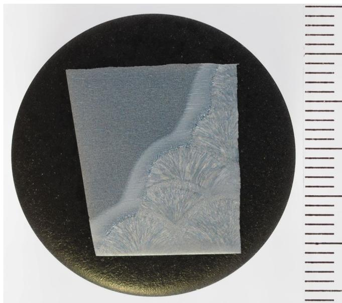
**Figure 4.3.** A specimen for general metallographic evaluation of the investigated weld. The sample is a corner cut from trepan 3 next to the inner surface of the trepan. The scale on the right edge has a line spacing of 1 mm.
