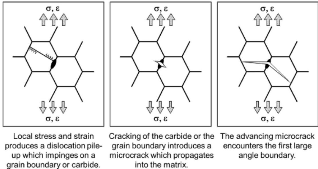
**Figure 3.3.** Schematic presentation of a typical cleavage fracture initiation process [44, p.116 Fig.4.2].
