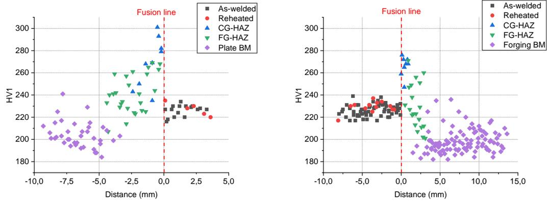
**Figure 5.4.** HV1 results with the fusion line at zero distance. On the left is the hardness profile from the plate base material to the HAZ and to the weld. On the right is the profile from the weld to the HAZ and to the forging. Observe the different length of the measurements across the fusion line compared to the HV10 measurements.
