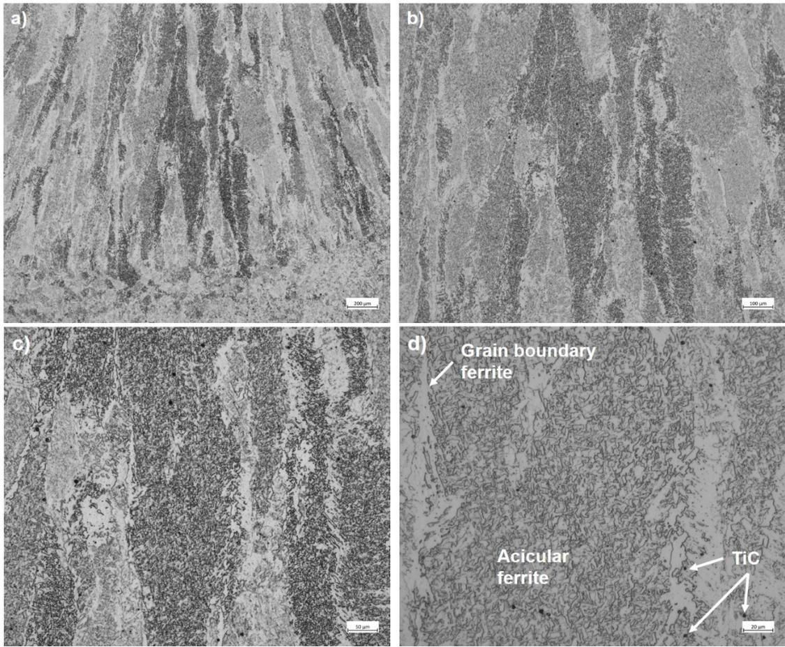
**Figure 5.18.** Darker-coloured weld bead microstructure at different magnifications. In the a) the bottom shows also reheated microstructure, and in the d) the titanium carbide (TiC) particles are seen as indicated by the arrows.
