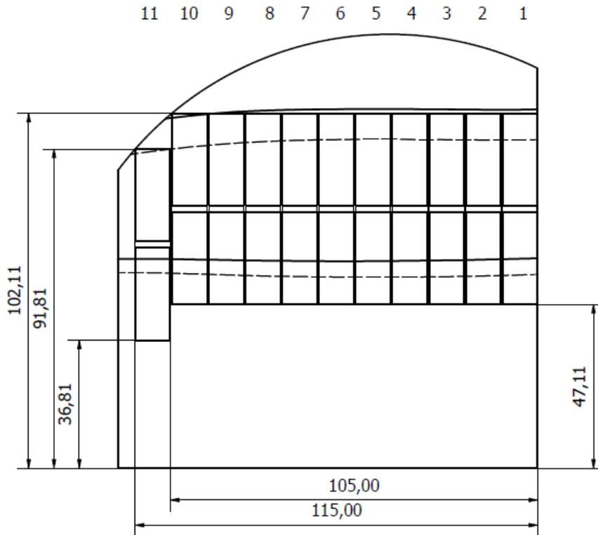
Figure 5. Cutting schematics for impact specimens from slice B of trepan 2. The identification number of each specimen is indicated so that the complete ID becomes B2B-XX, where XX is the number above.
