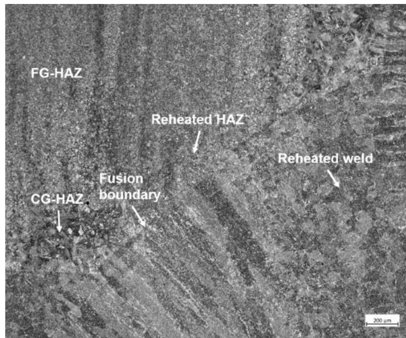
**Figure 5.11.** Fusion line of the outer weld beads with reheated regions.
