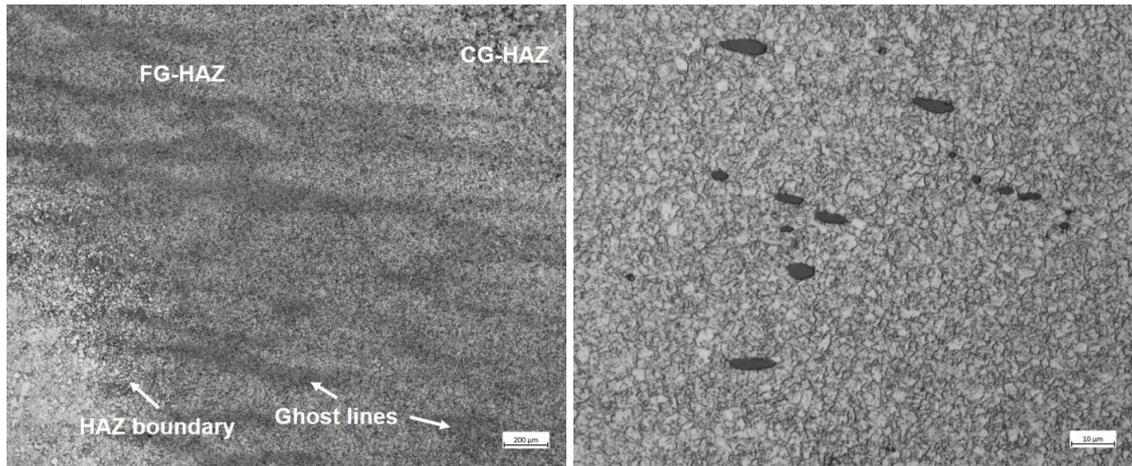
**Figure 5.16.** Fine-grained HAZ in the plate base material. In image on the right is the fine-grained HAZ with manganese sulphide (MnS) particles in the ghost line.
