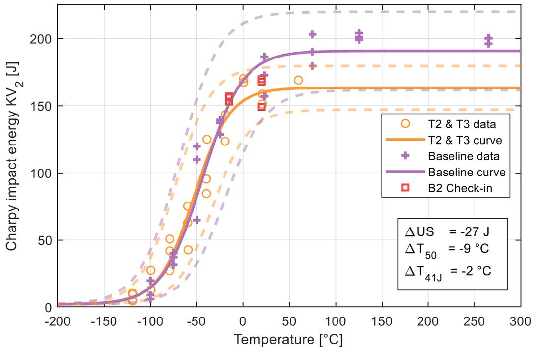
Figure 9. Comparison of transition curve of B2 RPV head SAW weld metal at  $\frac{1}{4}T$  from trepans 2 and 3 to the baseline data from [1] and its transition curve, determined using identical methodology as for the B2 weld. Additionally, B2 check-in data is also included. The changes in upper shelf energy  $C_{vUS}$ ,  $T_{50}$  and  $T_{41J}$  are also provided. It should be noted that B2 RPVH WM is not strictly identical to surveillance material.
