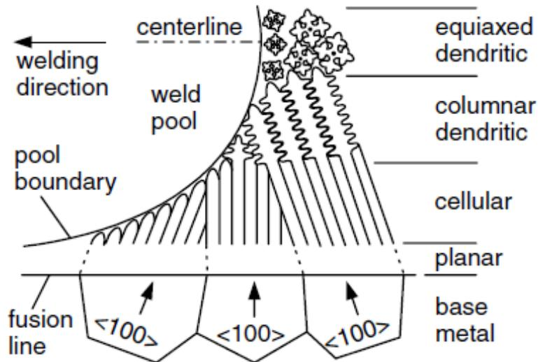
**Figure 2.5.** The solidification modes across the fusion zone behind the weld pool: planar, cellular, columnar dendritic, equiaxed dendritic. Additionally, the epitaxial growth is schematically shown. [10, p.202 Fig.8.5]
