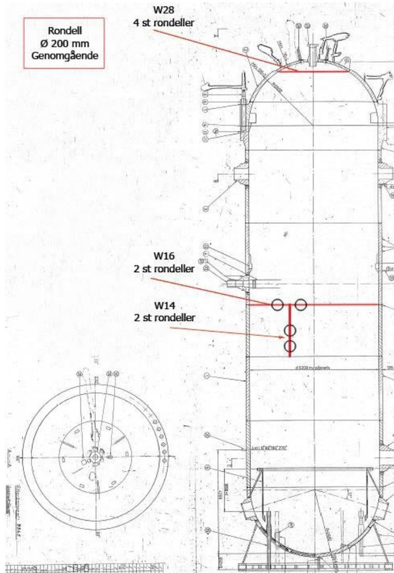
Figure 1. Schematic drawing of Barsebäck 2 RPV with W28 highlighted on the top. Beltline welds, from which trepans have also been extracted, are also marked. [3]
