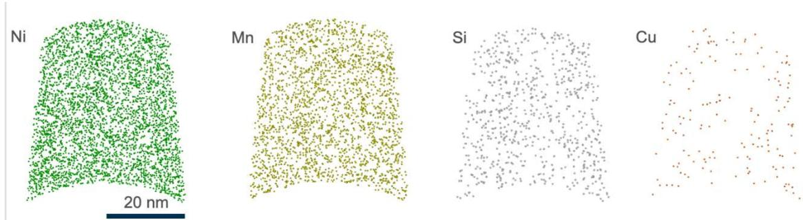
Figure 1. 5 nm thick slices from the APT reconstruction of the analysis of the irradiated material. No clusters are observed.
