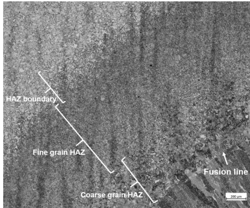
**Figure 5.7.** The heat-affected zone regions in the forging base material.
