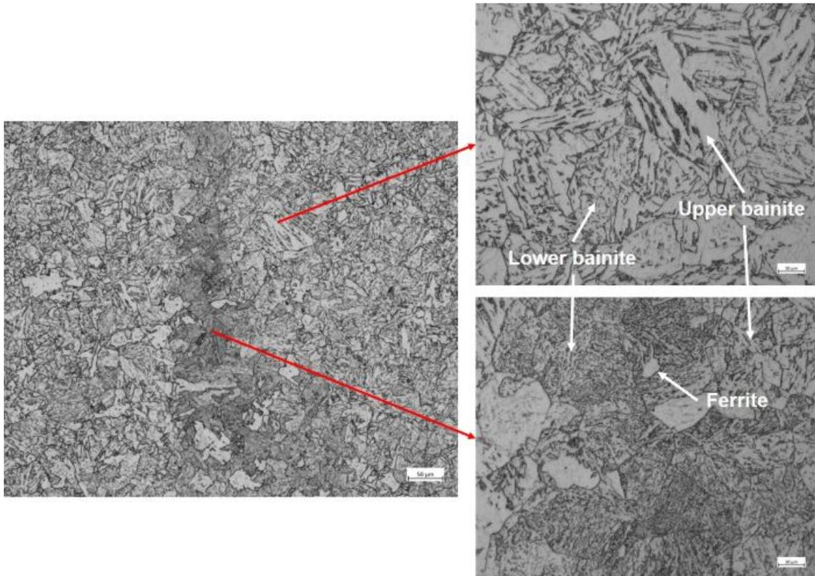
**Figure 5.6.** Bainitic forging base material. The ghost line is shown in the micrograph on the left. In the two figures on the right, the microstructures of the typical base material and the ghost line are shown at a higher magnification.
