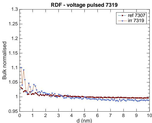
Figure 2. The Ni-Ni radial distribution function (RDF) of the irradiated material, compared with the reference material. A normalised value higher than 1 for short distances implies tendencies towards clustering of atoms.
