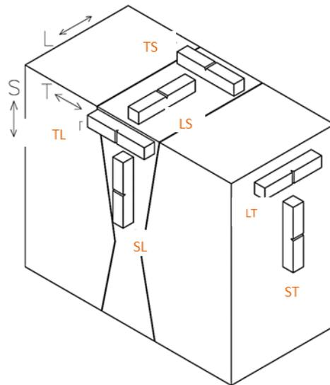
Figure 2. Picture showing orientations of specimens in weld metal and base material. T-S was used for the weld metal impact test specimens.
