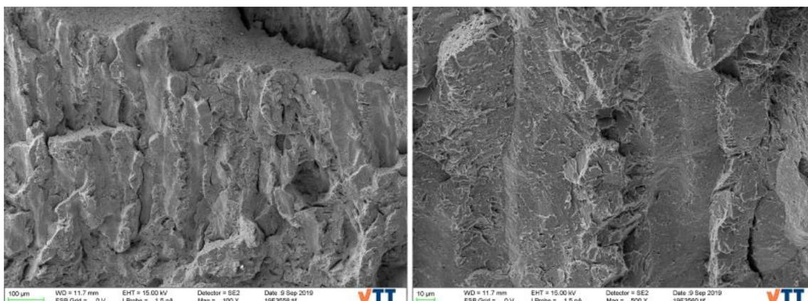
**Figure 6.1.** Interdentritic and intergranular fracture in the as-welded microstructure of a brittle fracture specimen.
