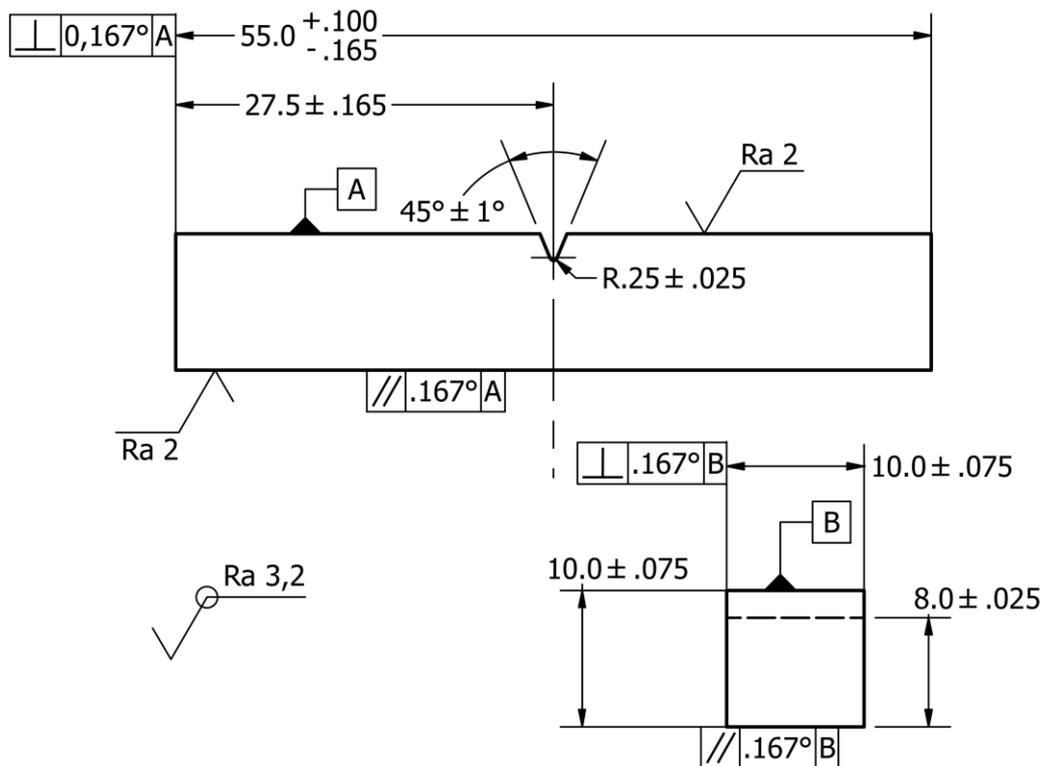
Figure 4. An illustration of a Charpy-V impact specimen along with the dimensional requirements. All measures are in millimetres unless implied otherwise.
