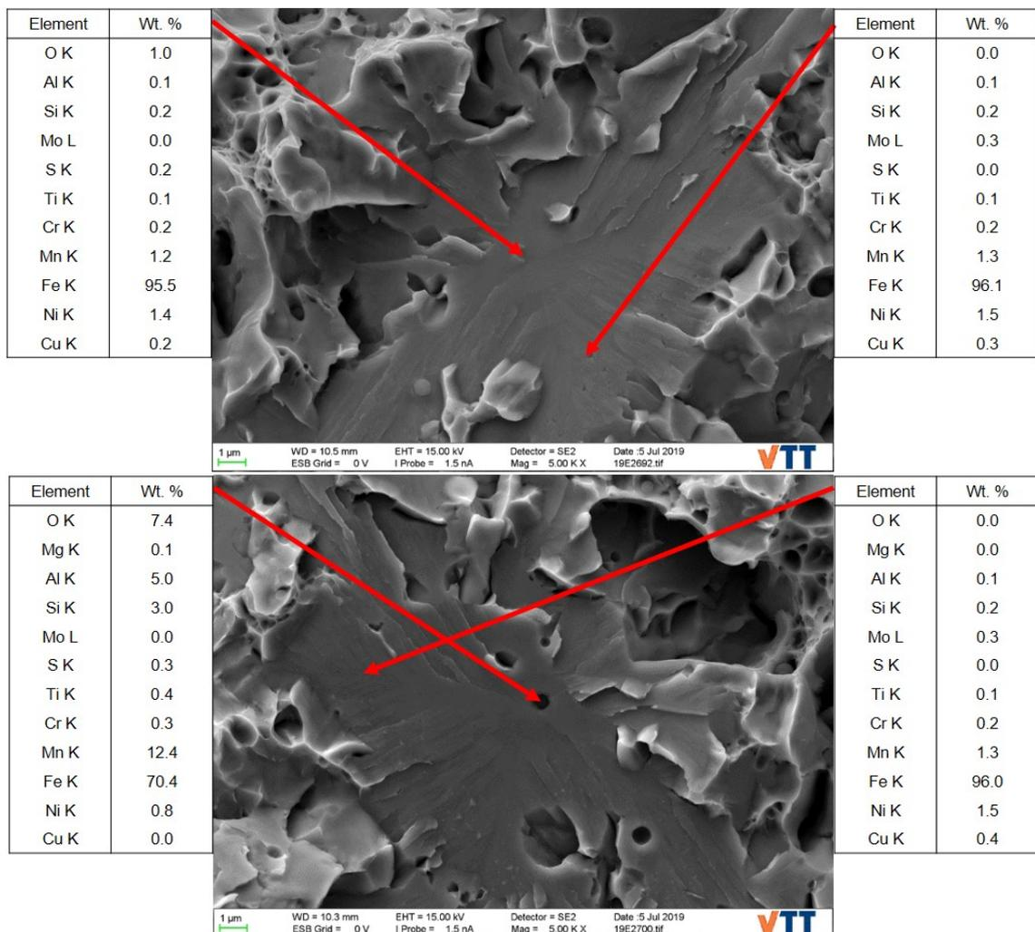
**Figure 5.23.** Semi-quantitative chemical compositions (wt%) obtained by EDS point analysis of specimen CVN 8, half A on top and half B on bottom. On the left is shown the composition of the primary initiation site and on the right the composition of the surrounding matrix.
