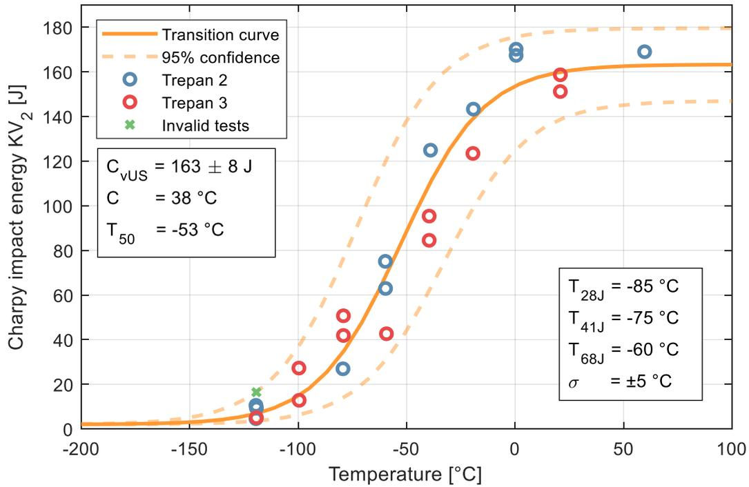
Figure 8. Impact transition curve for B2 RPV head SAW weld metal at  $\frac{1}{4}T$ , extracted from BRUTE trepans 2 and 3.
