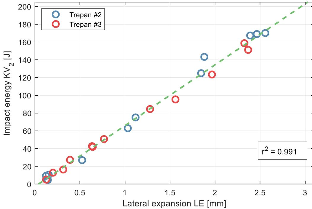
Figure 11. Impact energy  $KV_2$  in relation to lateral expansion  $LE$ . A linear regression model is fitted to the data.
