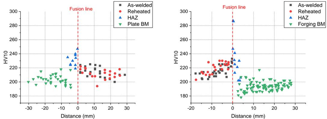
**Figure 5.3.** HV10 results over the weld. On the left is the hardness profile from the plate base material to the HAZ and to the weld. On the right is the profile from the weld to the HAZ and to the forging base material. The fusion line is set at the zero distance.
