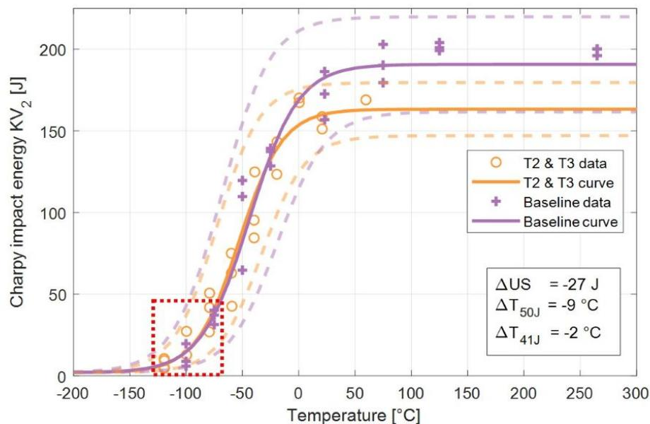
**Figure 6.2.** Transition curves from the experiments on T2 and T3 (trepan 2 and trepan 3) with a comparison to the baseline curve obtained in a surveillance program. The red box contains the data points used in the brittle fracture characterisation.
