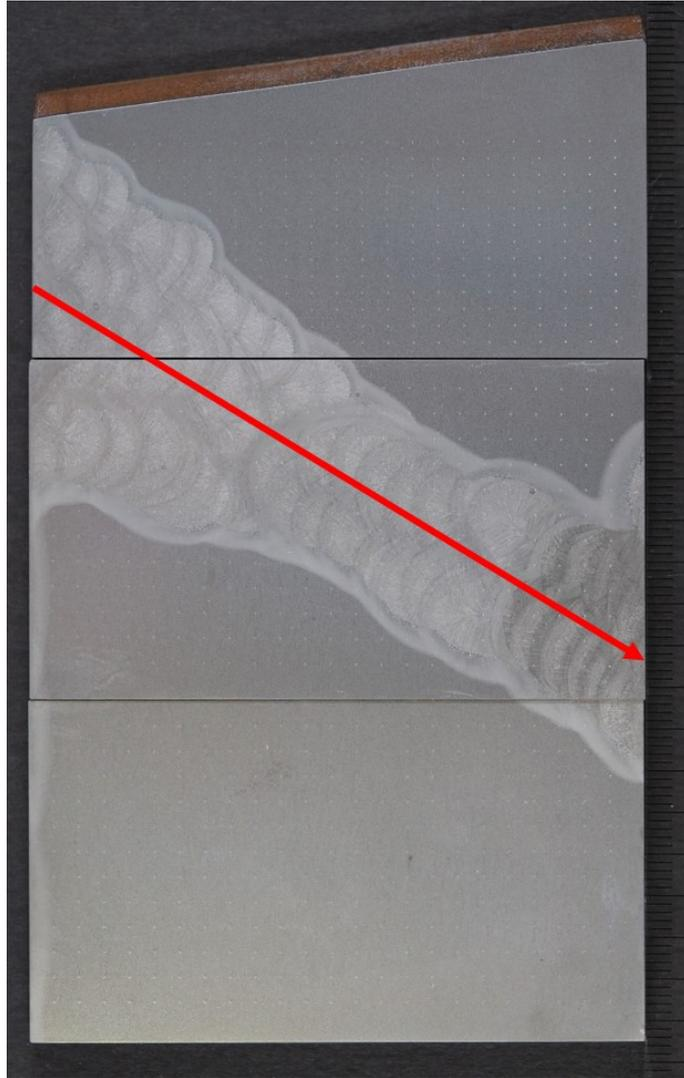
**Figure 5.1.** HV10 profile direction through the weld build-up thickness from the inner wall to the outer wall. The plates from bottom to top are numbered as 3S1, 3S2, and 3S3. The scale on the right edge has a line spacing of 1 mm.
