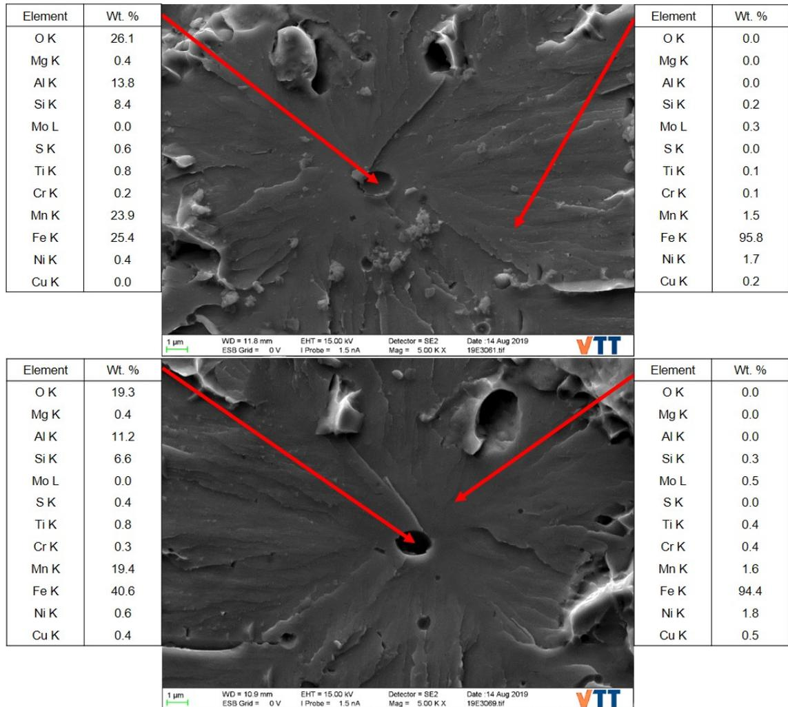
**Figure 5.29.** Semi-quantitative chemical compositions (wt%) obtained by EDS point analysis of specimen CVN 2B5, half A on top and half B on bottom. On the left is shown the composition of the primary initiation site and on the right the composition of the surrounding matrix.
