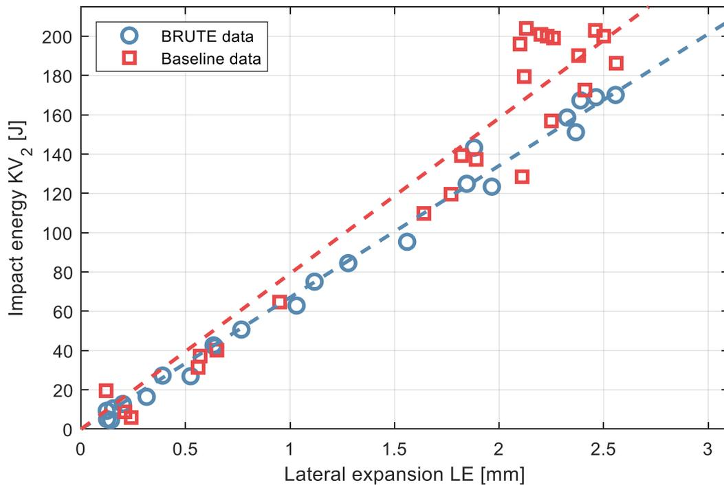
Figure 12. Impact energies  $KV_2$  and corresponding lateral expansions  $LE$  from baseline data [1] and test results of B2 RPV head SAW weld metal at  $\frac{1}{4}T$  from trepans 2 and 3. Linear model are fit to both datasets separately with intersections bound at origin.
