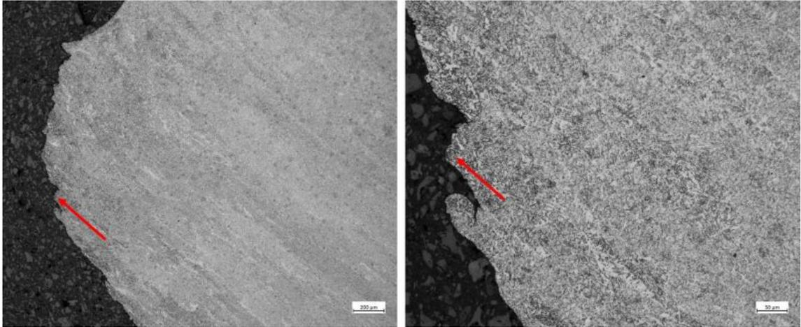
**Figure 5.26.** *Microstructure of the cross-section specimen CVN 8. The arrows point to the approximate location of the primary initiation site on the fracture surface.*
