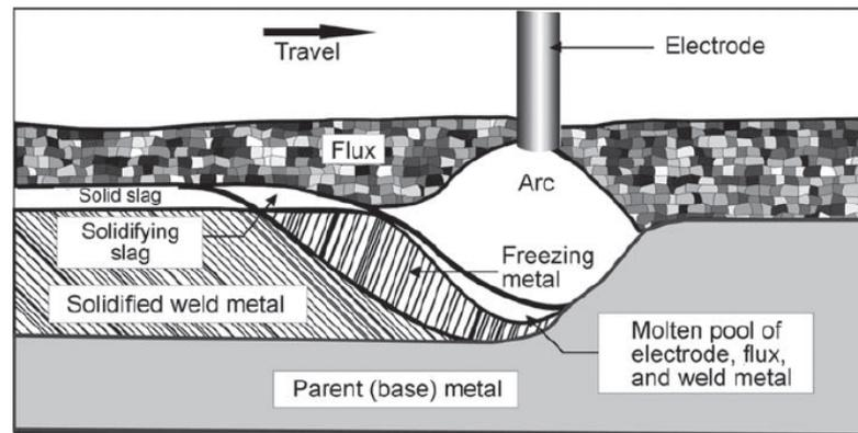
**Figure 2.1.** Principle of the submerged arc welding and the weld pool formation. [11, p.335 Fig.2]
