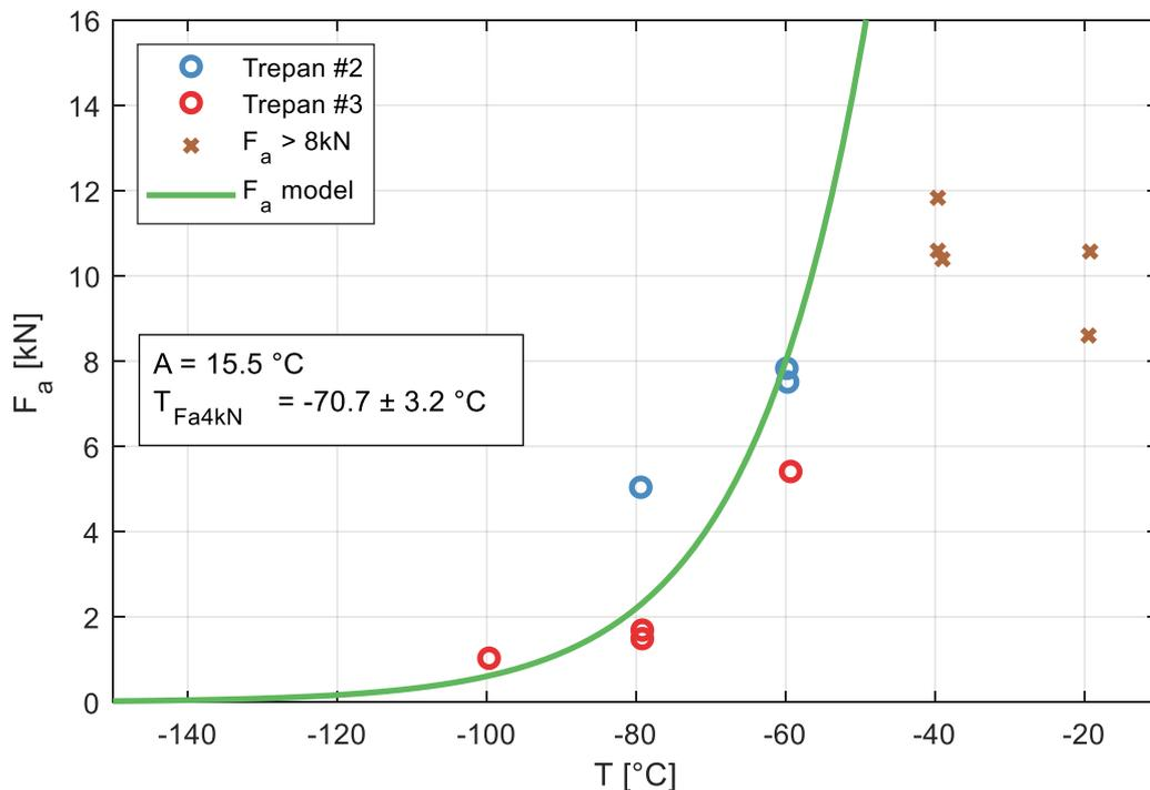
Figure 10. Crack arrest force data and exponential model for the B2 RPV head SAW weld metal at  $\frac{1}{4}T$ . Only circled values are used in the model. The model uses fitting parameters  $A$  and  $T_{F_{a4kN}}$ , of which  $T_{F_{a4kN}}$  is the transition reference temperature of  $F_a$ .
