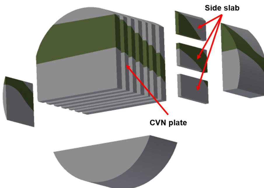
**Figure 4.1.** All major cuts of trepan 3 are shown, including the plate where all the CVN specimens are cut and the side slab that is cut into three pieces. The weld is seen as darker colour in the middle.
