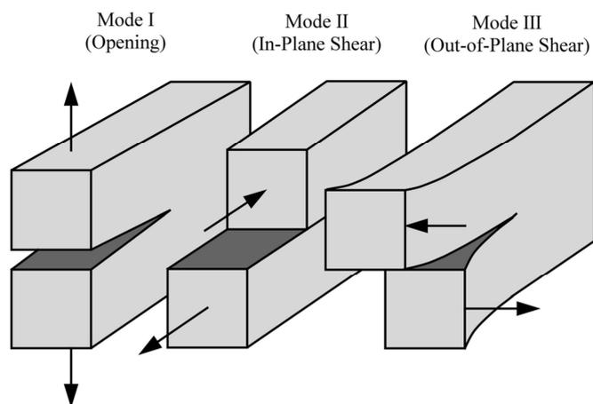
**Figure 3.1.** *The three failure modes presented schematically [32, p.43 Fig.2.14]*
