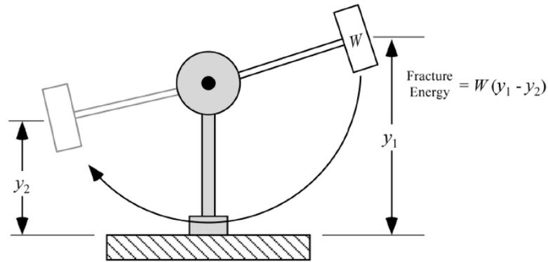
**Figure 3.6.** Principle of the pendulum device used in the Charpy-V impact testing. The fracture energy is obtained from the weight of the cross-head and the height difference of the pendulum. [32, p.342 Fig.7.21].
