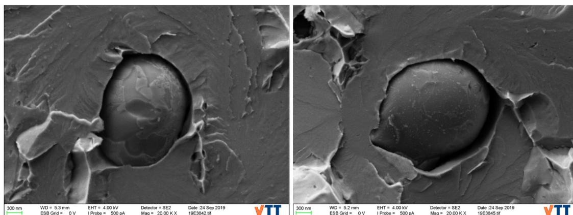
**Figure 6.3.** Particle at the primary initiation site in specimens CVN 9 and CVN 2B7. The particle sizes in this case are approximately 1.5  $\mu\text{m}$  and 2.5  $\mu\text{m}$ , respectively.
