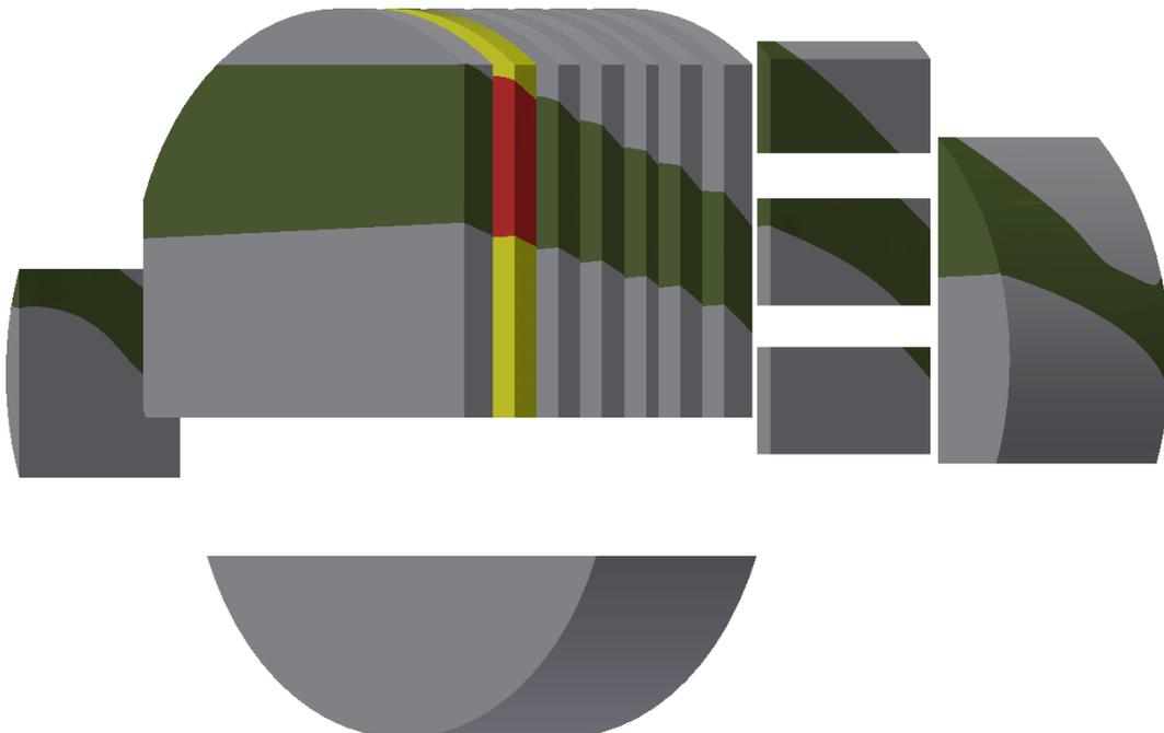
Figure 3. The main cuts of trepan 3. The tensile specimens from  $\frac{1}{4}T$  depth are fabricated from slice B that is highlighted in red and yellow.
