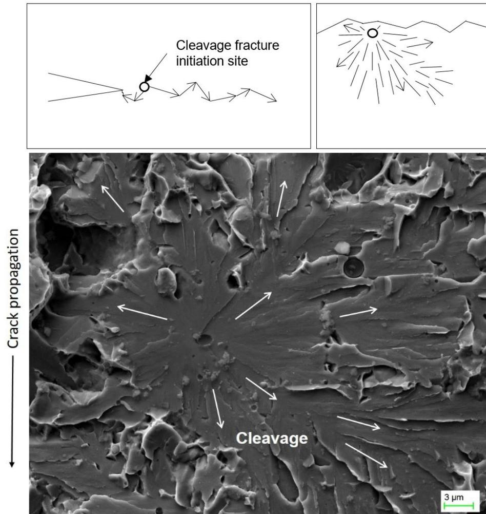
**Figure 3.4.** Cleavage fracture initiation and propagation.
