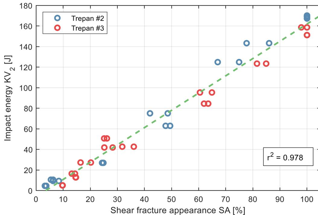
Figure 13. Impact energy  $KV_2$  in relation to shear fracture appearance SA. A linear regression model is fitted to the data.
