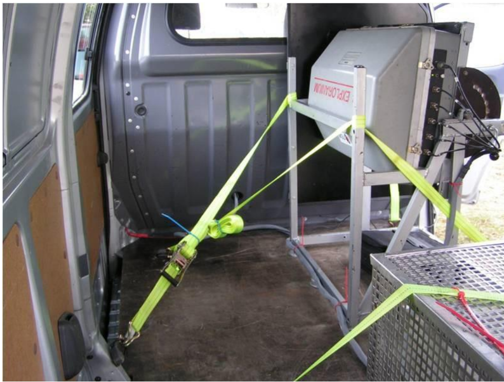
Figure A4-1: Placement of the detector system in the vehicle. The above picture is from an earlier exercise with an older system, but the placement of the RSX5 throughout MOMORC was similar.
