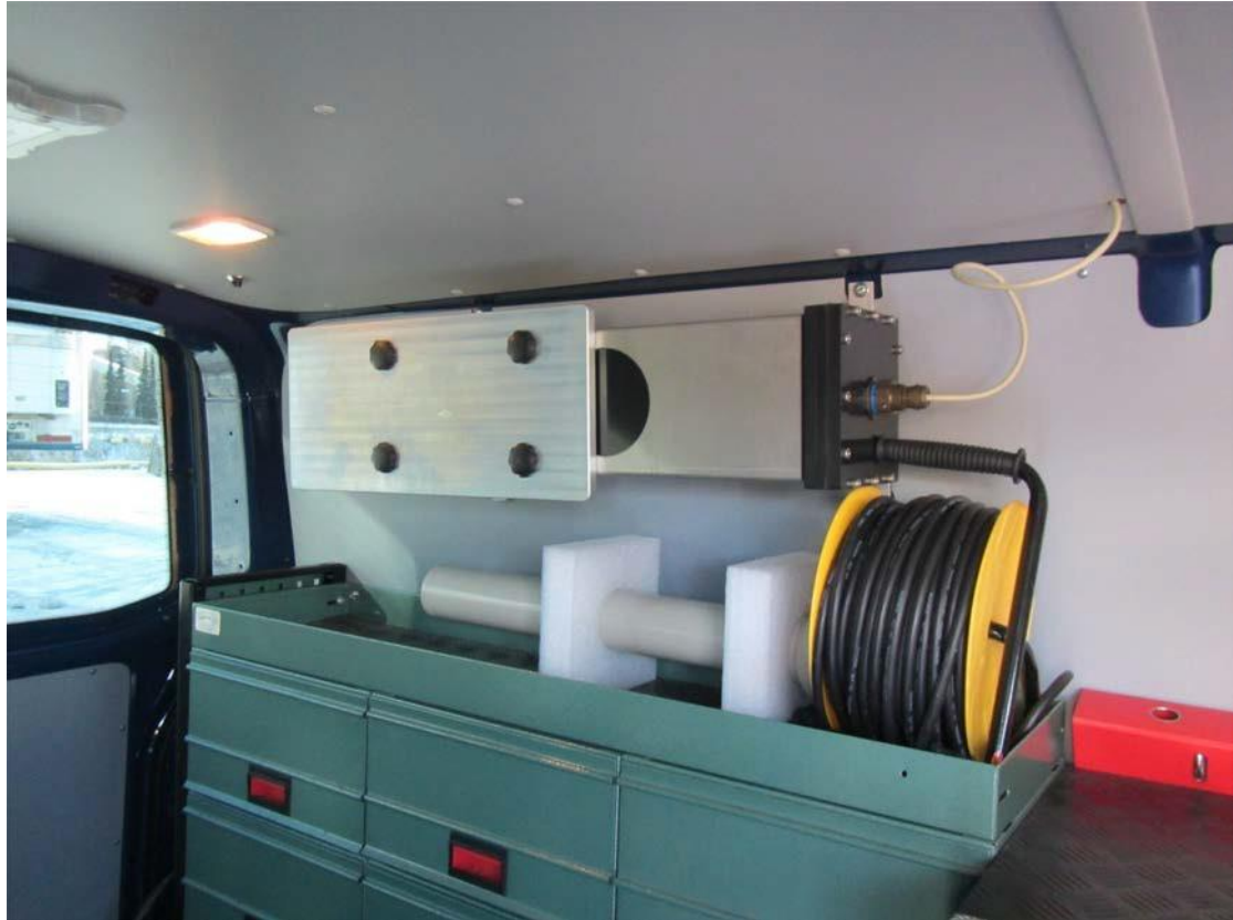
Figure A2-2. Detector mounting in detail. Removable steel plate covers the part of the housing where the detector is located.
