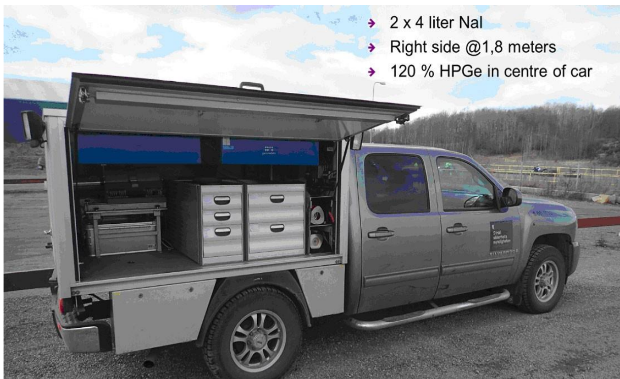
Figure A7-1. Detector set-up in the SSM Chevrolet Silverado.
