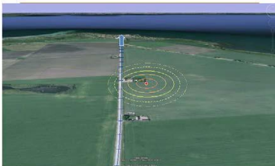
Fig 2.2 Schematic principle of mobile detection of point sources when driving along a road. Data acquisition is divided into time slots. The source can be detected in one or more time slots.
