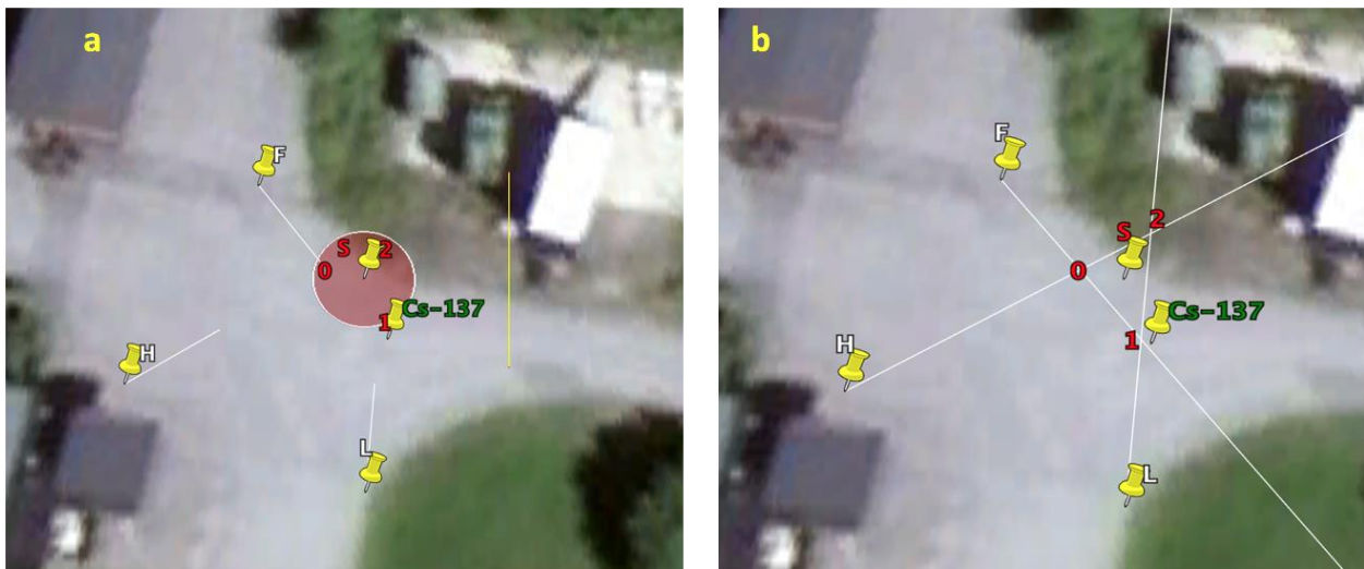
Figure 2 ^{137}\text{Cs} source (1.7 GBq) localized using three measurements (FHL). (a) The analyzed point of location (S) is 3.1 m from the true source location labelled as ^{137}\text{Cs} . For reference, the length of the yellow line is 10 m. The mean-deviation circle has a radius of 2.4 m. (b) Original RandidSOLO localization vectors.
