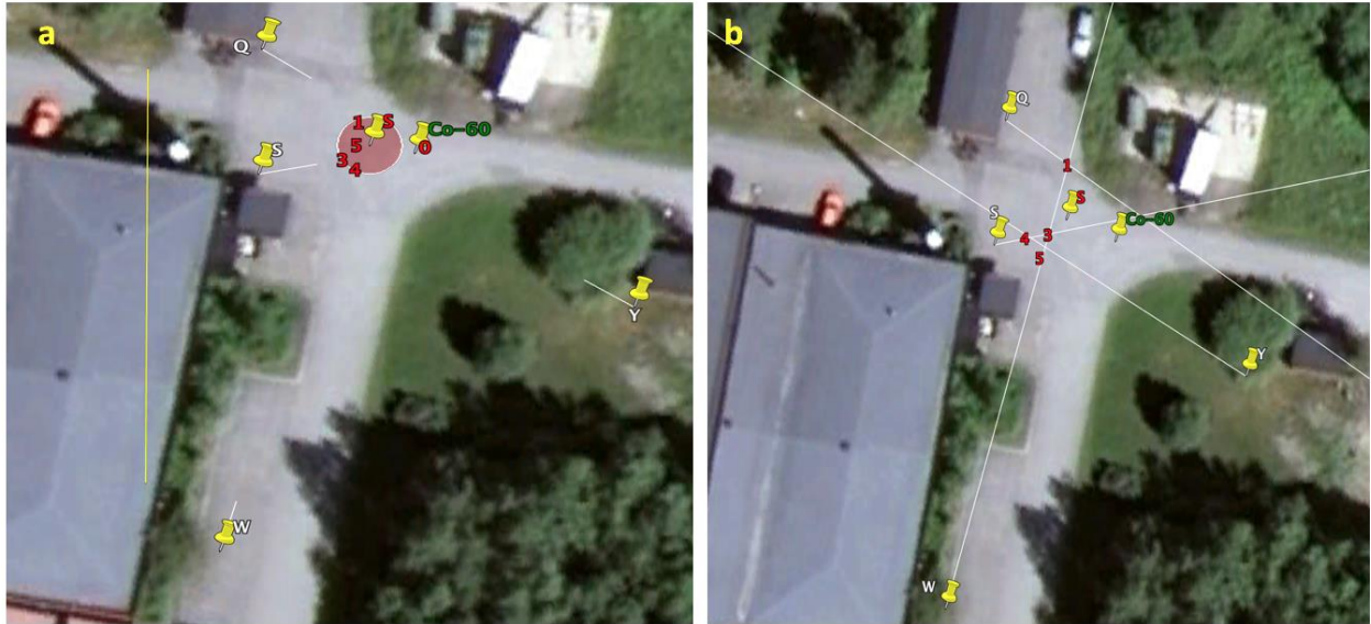
Figure 3 ^{60}\text{Co} source (4.3 GBq) localized by four measurements (QSYW). (a) The analyzed point of location (S) is 3.8 m from the true source location labelled as ^{60}\text{Co} . For reference, the length of the yellow line is 40 m. The longest source-detector distance is 41.2 m (WS) and the mean-deviation circle has a radius of 2.6 m. (b) Original RanidSOLO localization vectors.
