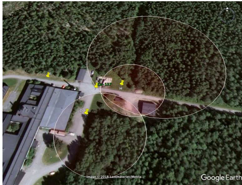
Figure 1 ^{137}\text{Cs} source localization based on cps-ratios. Air absorption correction was performed iteratively by hand calculations. Difference between true and estimated location is 6.9 m.
