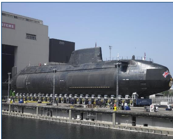
A British SSN Astute class submarine ready for launch. The class has a 7,400 t submerged displacement. Source: Defence. Industry Daily.
