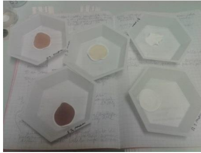
Figure 6. \text{SrCO}_3 precipitations obtained after filtration in UH-Sr-I and UH-Sr-II methods for IAEA-TEL-no.5 soil. Three rust-colored precipitations (left) are the soil samples, two white-colored are blanks (right).
