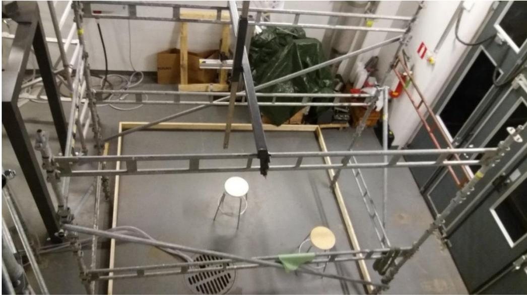
Figure 2. The spray testing station with the support structure and the wooden rail.
