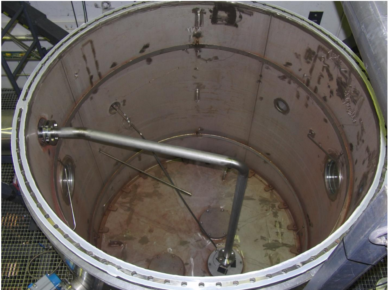
Interior of the try well compartment and DN65 steam line.
