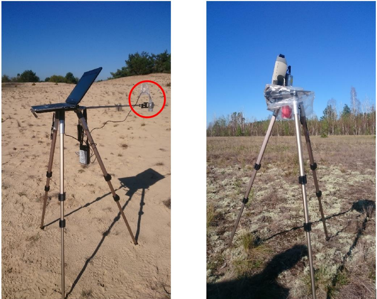
Figure 5. Detector systems used by the NRPA during GAMFAC exercise. Left: The CZT detector setup at Site 2 (red circle), together with the dose rate meter (hanging from the tripod). Right: NaI detector setup at Site 1.
