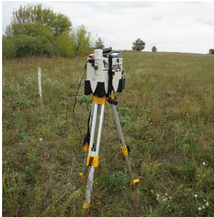
Figure 9. The Ortec Detective EX High Purity Germanium detector employed by the Swedish team.
