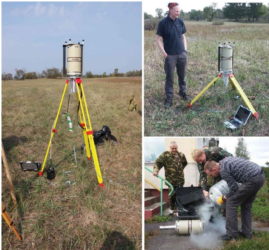
Figure 20. The Icelandic team detector in two height configurations (left and top right) and while filling liquid nitrogen (bottom right).
