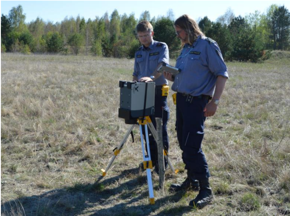
Figure 11. The Canberra Falcon Ge-detector mounted on a tripod at Site 1.
