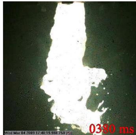
Figure 5. The melt jet injection in the TS-3 experiments at two different times.[HONG et al. (2009b)]
