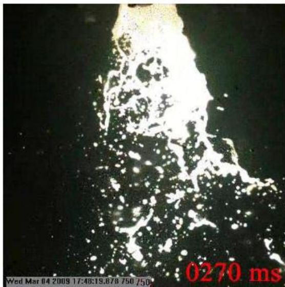
Figure 5. The melt jet injection in the TS-3 experiments at two different times.[HONG et al. (2009b)]
