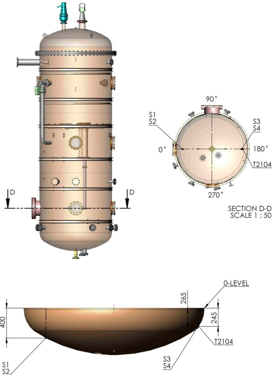
*Strain gauges and thermocouple T2104 on the outer wall of the pool bottom.*
