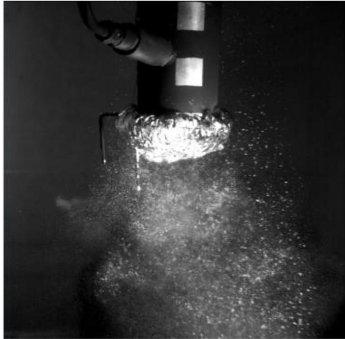
Figure 10. Steam release into subcooled water in the PPOOLEX test facility.
