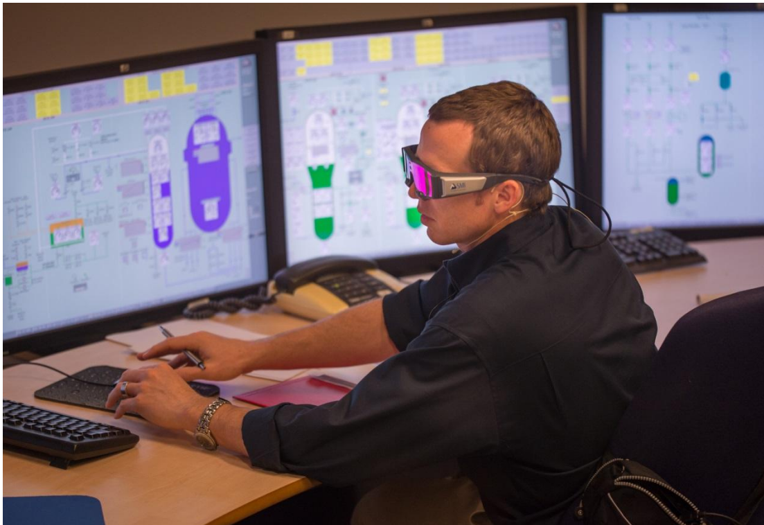
Figure 10. Participant in the resilient procedure use study wearing eye tracking glasses with a built-in scene camera.
