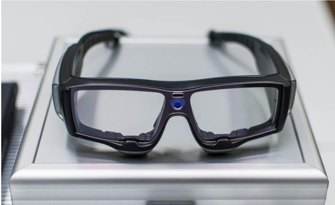
Figure 13. Close-up view of the SMI Eye Tracking Glasses used in this study. The hole in the nose bridge of the glasses houses the scene camera.
