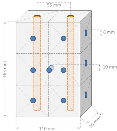
**Figure 3.** Drawing of a fully-sized scatterer. Half blocks have a thickness of 25 mm instead of 55 mm. Source tubes are presented by orange cylinders. The blue dots are connector-holes with a depth of approximately 10 mm.
