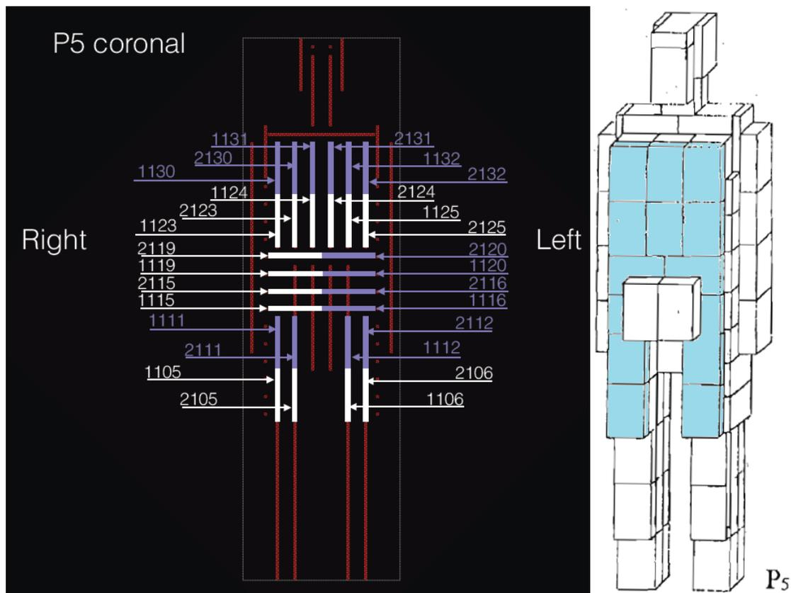
Figure 9: Excerpt from file “P5.pdf” (pg. 3) to demonstrate material ID mapping of scatterers in 2<sup>nd</sup> y-plane.
