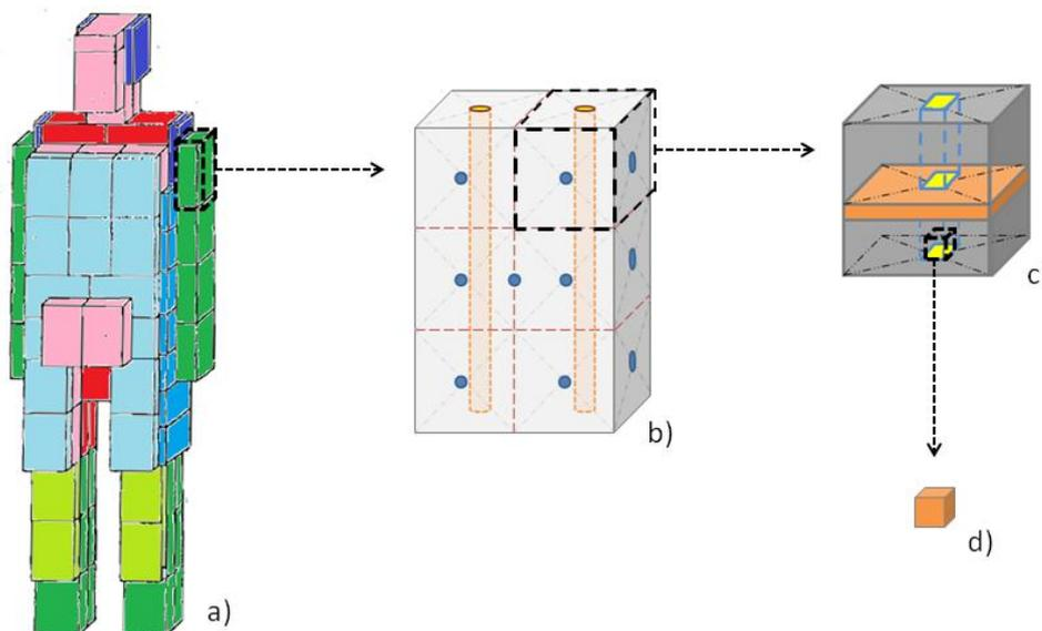
**Figure 4.** a) IRINA\_P5 made up of, b) scatterers made up of, c) unit cubes made up of, d) voxels.
