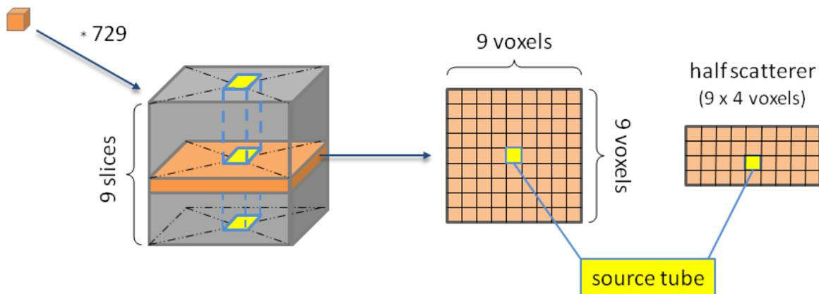
**Figure 6.** Sketch of how to build a unit cube, used to compose a fully-sized scatterer. 729 voxels build one cube: 9 slices à  $9 \times 9$  voxels. No connector-holes; only *square* source tube in the middle. (One slice of a half scatterer with  $9 \times 4$  voxels with central source tube in the third row.)
