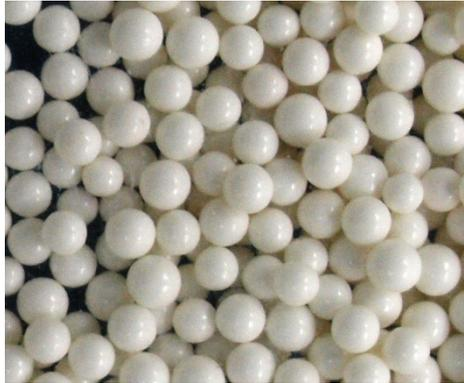
*Fig. 3. Ceramic beads used as debris simulant.*
