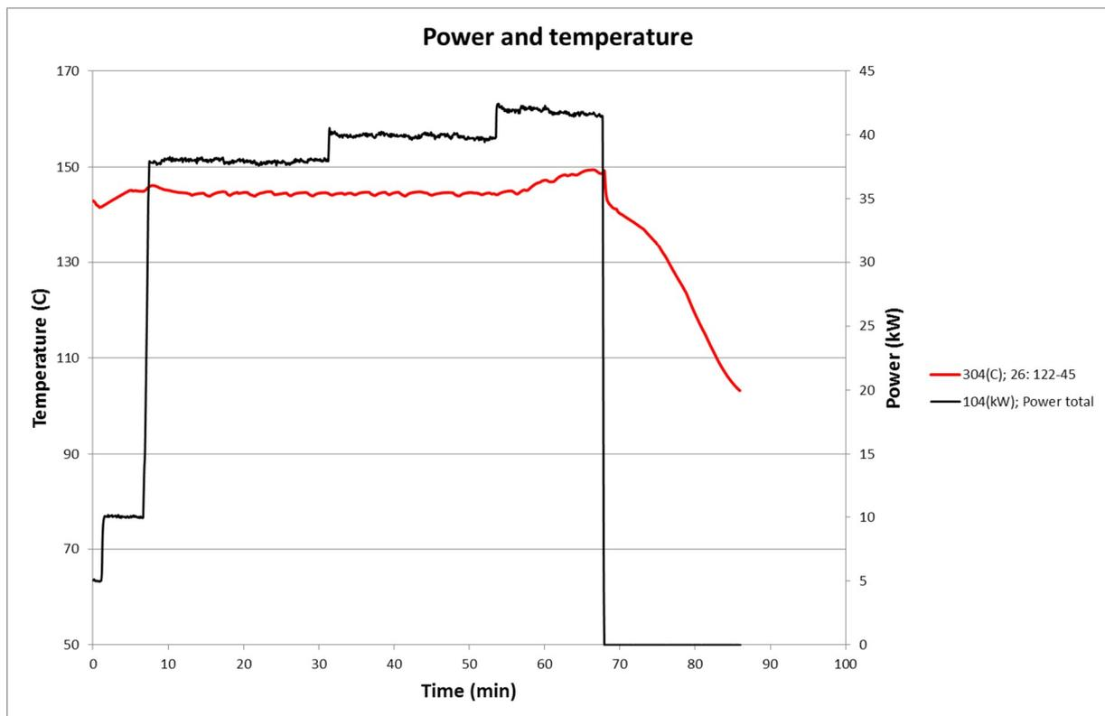
Fig. 10. Control power and the temperature of the sensor indicating dryout in COOLOCE-11d.
