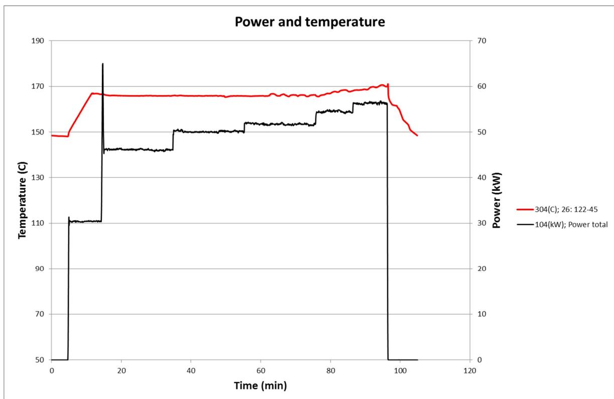
Fig. 14. Control power and the temperature of the sensor indicating dryout in COOLOCE-11f.
