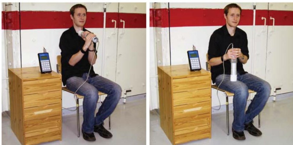
Figure 9: Illustration for thyroid and corresponding background measurement, as recommended in TMT handbook (Rojas-Palma et al., 2009)
