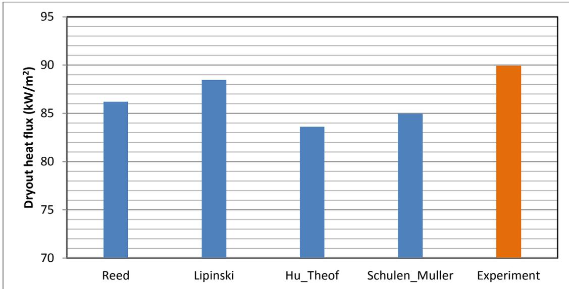
Fig. 10 Comparison of the dryout heat flux in Bed-1 with various models under top flooding conditions
