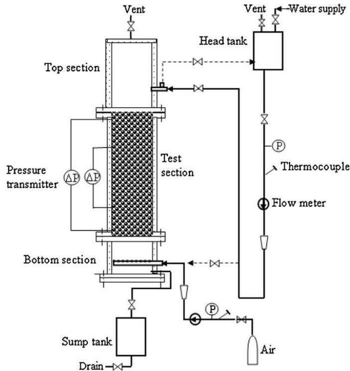
Fig. 1. Schematic of POMECO-FL facility
