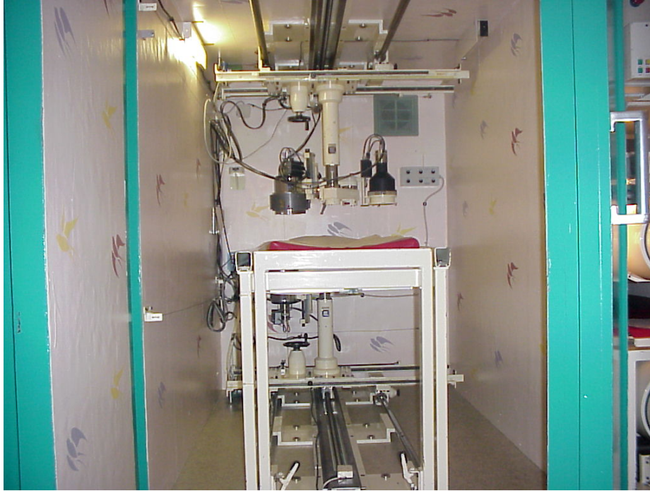
Figure 6. NaI-system at the Dept. of Radiation Physics, University of Gothenburg (picture courtesy of Mats Isaksson, Prof., Radiation physics, University of Gothenburg)
