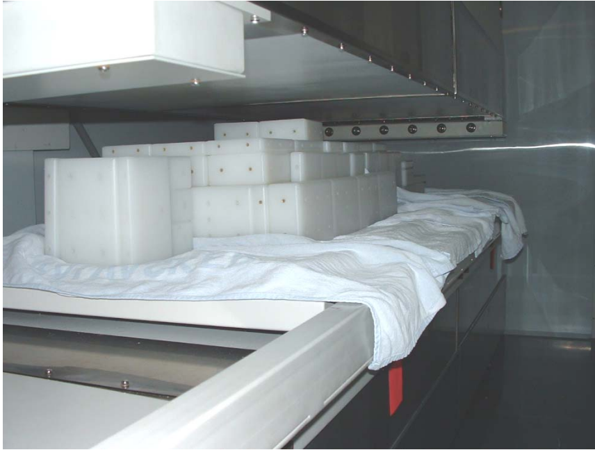
Figure 8. Counting system 1 with plastic scintillators at Rigshospitalet in Copenhagen; the phantom IRINA m lies in the bed for the PIANOLIB measurements (picture courtesy of Holger Jensen and Soren Holm, PET Rigshospitalet)
