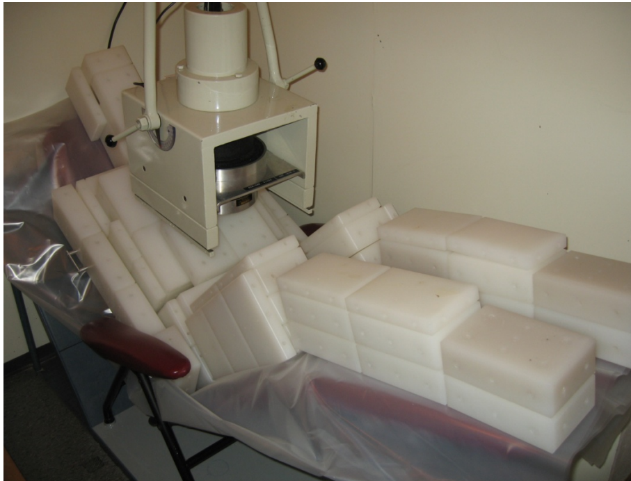
Figure 7. Measurement set up for the PIANOLIB exercise at the Institutt for energiteknikk, Kjeller (picture courtesy of Ann-Helen Haugen, Health and Safety Dept., IFE Kjeller)
