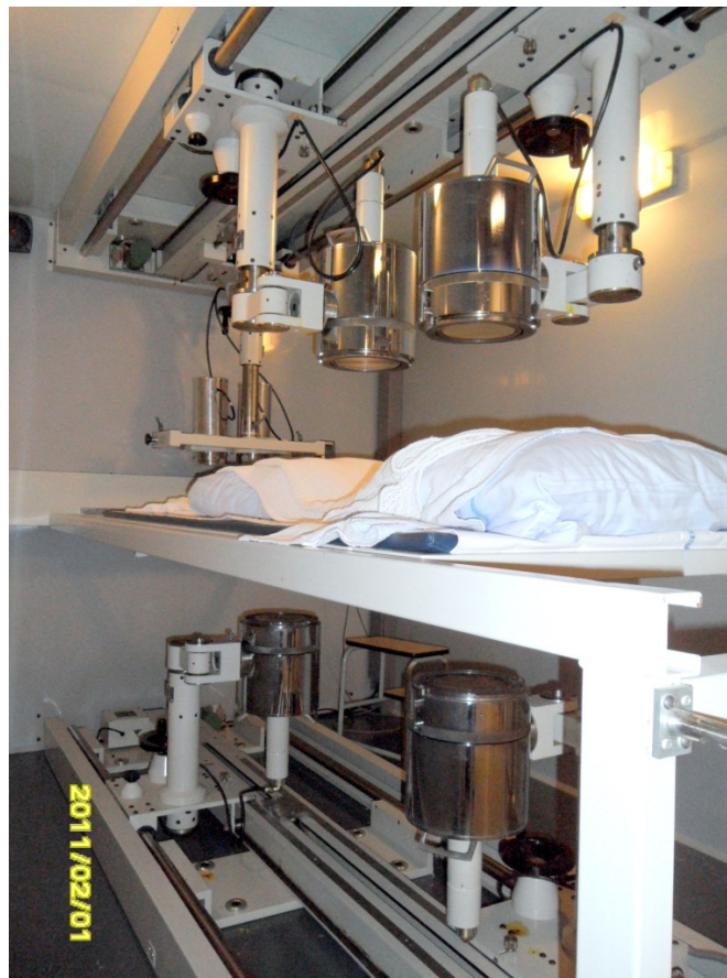
Figure 9. Counting system 2 with NaI crystal scintillators at Rigshospitalet in Copenhagen (picture courtesy of Holger Jensen and Soren Holm, PET Rigshospitalet)
