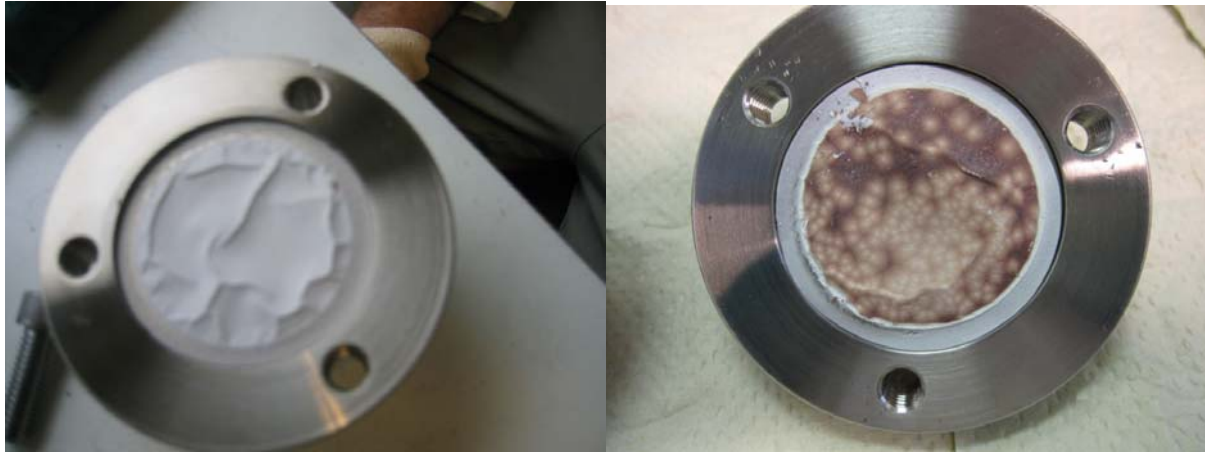
Figure 9. Pictures of the filter holders after two experiments. The holder to the left was used at dry conditions, while the holder to the right was used at humid conditions.
