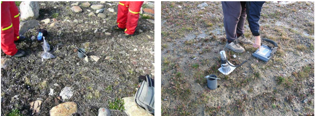
Figure 1: Soil collection at Thule (left) and gamma screening of soil using a portable NaI-detector (right).
