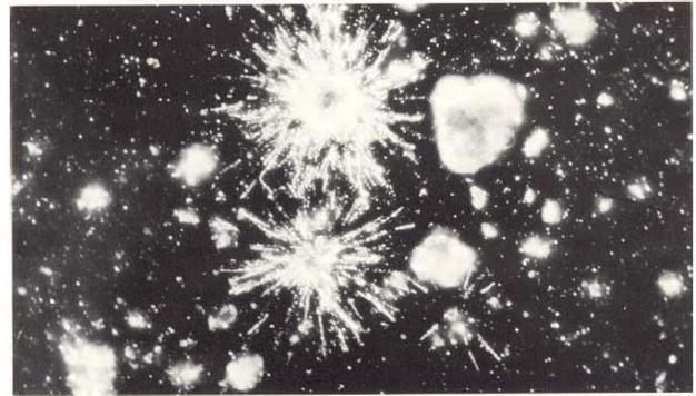
Figure 5. Microphotograph showing alpha tracks from plutonium particles in a sample from the crushed ice.
