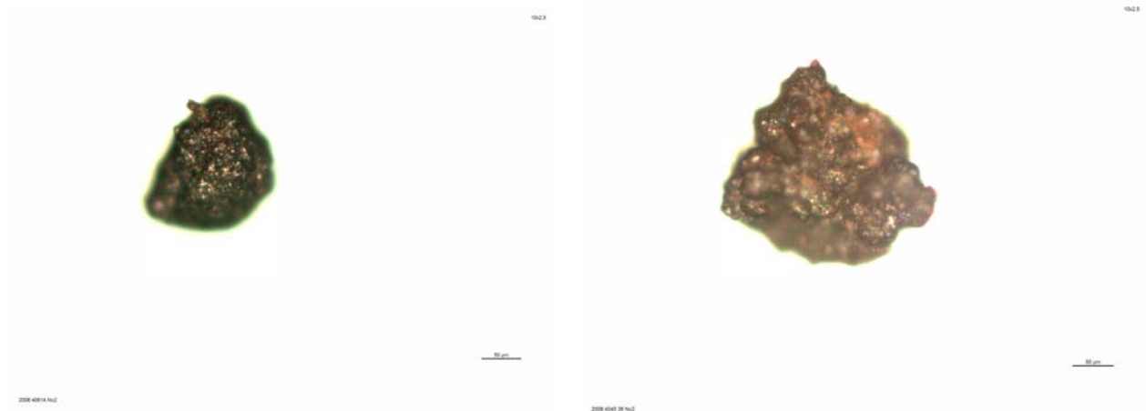
Figure 5. Optical microscopy pictures of two larger Thule actinide particles (fragments). Size of particles can be determined from the 50 \mu\text{m} bar in the pictures.
