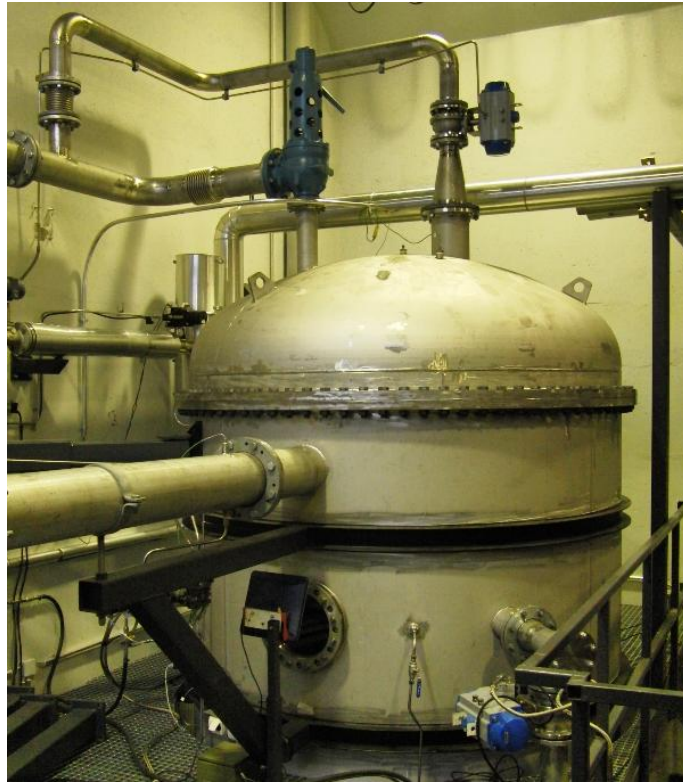
Dry well compartment, relief valves and inlet plenum.
