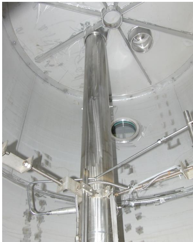
Inside view of the wet well compartment: blowdown pipe and intermediate floor.
