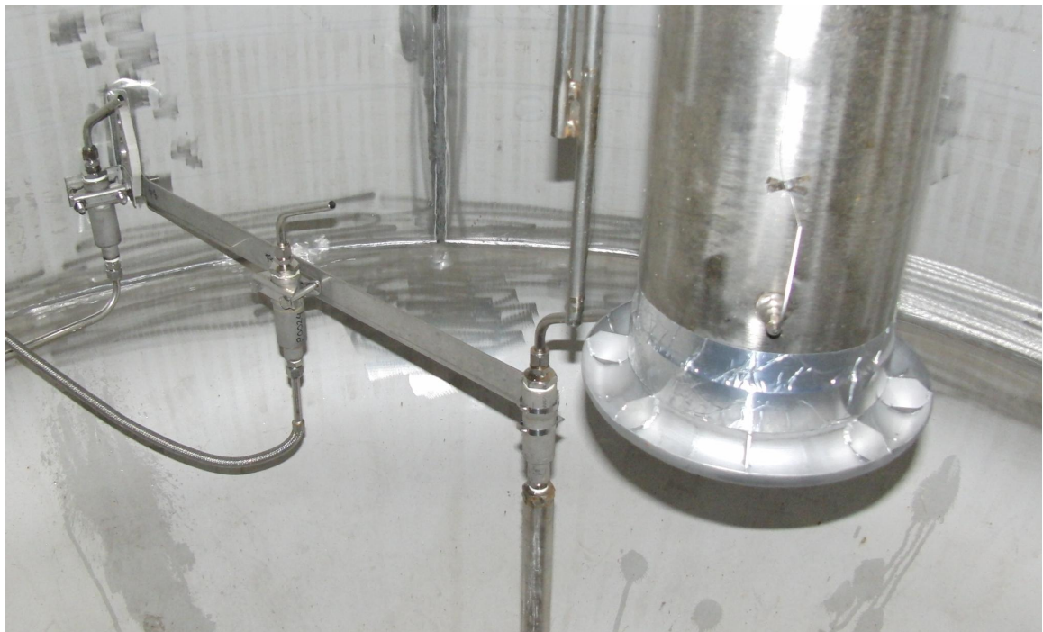
Pressure (P1, P5, P7 and P8) and temperature (T1 and T5) measurements at the blowdown pipe outlet.
