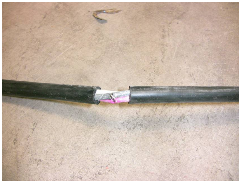
Figure 9 TXM1 cut on the insulation of 2 wires (dry)
