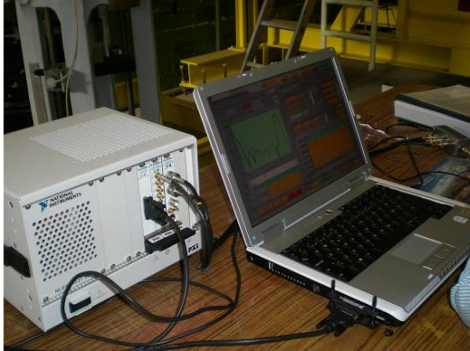
Figure 6: LIRA Generator, LIRA modulator and computer used in the tests
