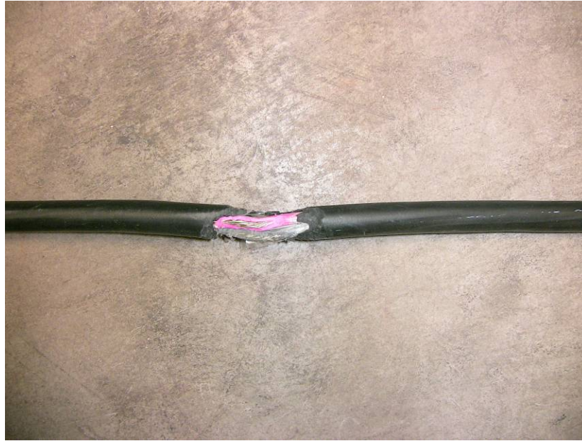
Figure 8 TXM2 gouge of 2 wires (dry)
