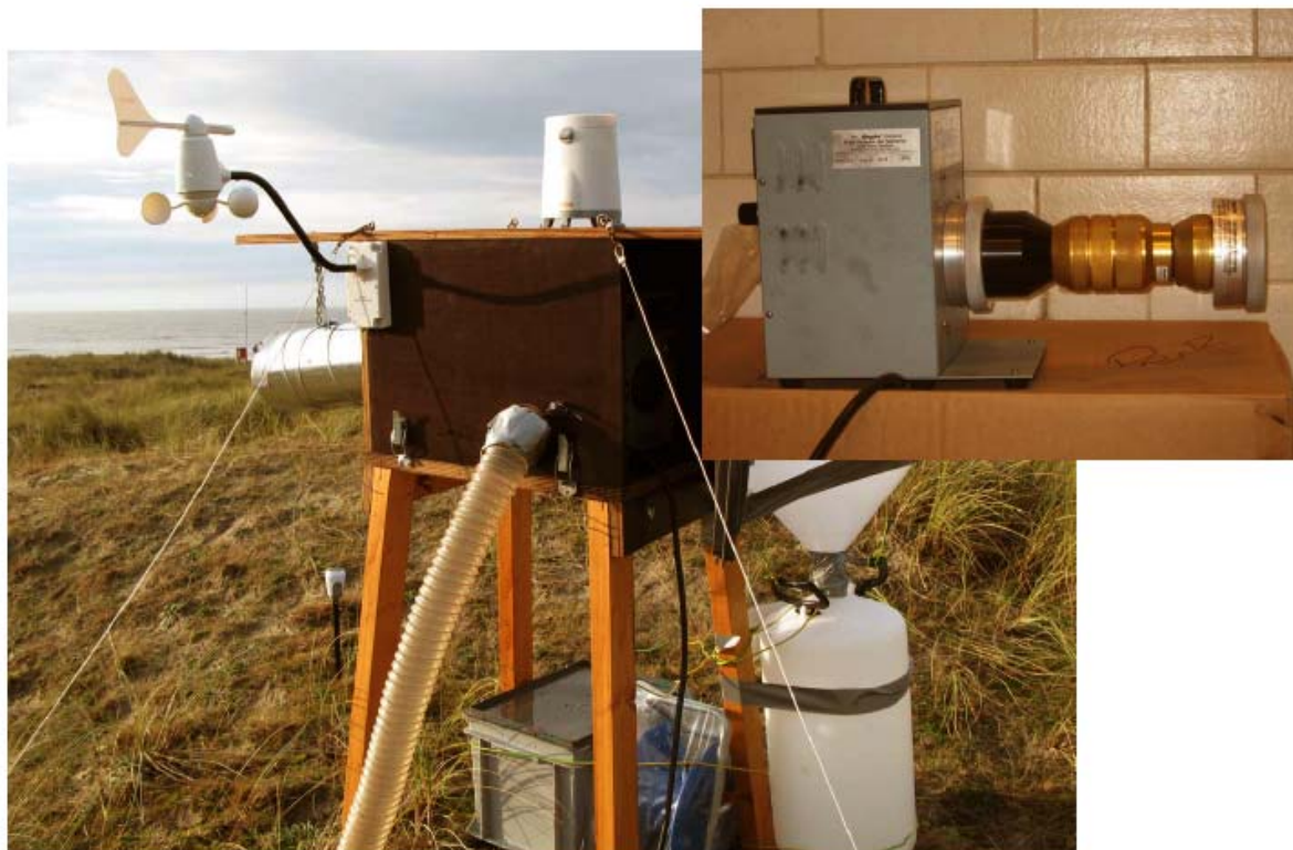
Fig.3 Air sampler for collected different species of iodine from atmosphere
