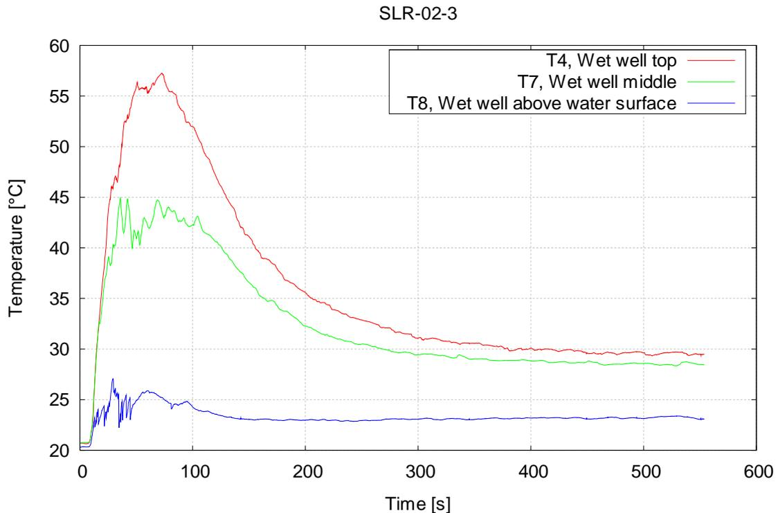
Figure 7. Temperatures in the wet well gas space in SLR-02-3.
