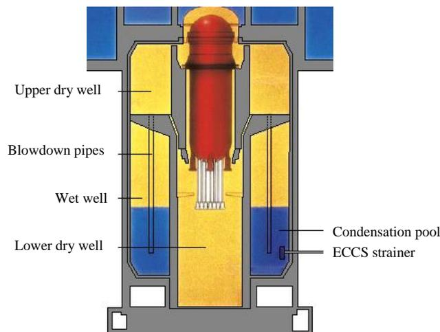
*Figure 1. Schematic of the Olkiluoto type BWR containment.*
