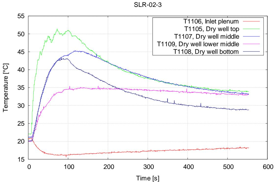
Figure 6. Temperatures in the inlet plenum and in the dry well in SLR-02-3.
