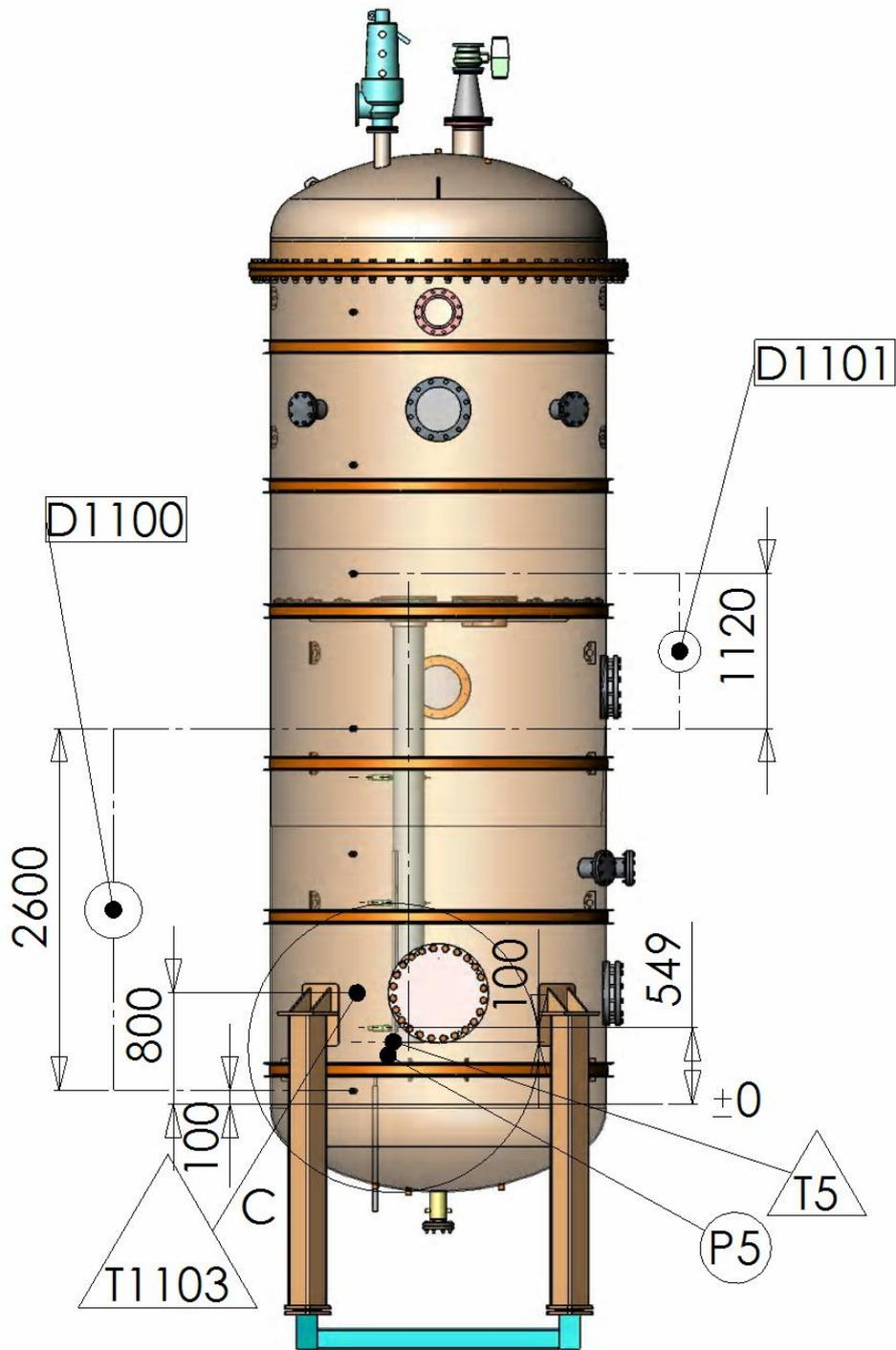
*Test vessel measurements.*
