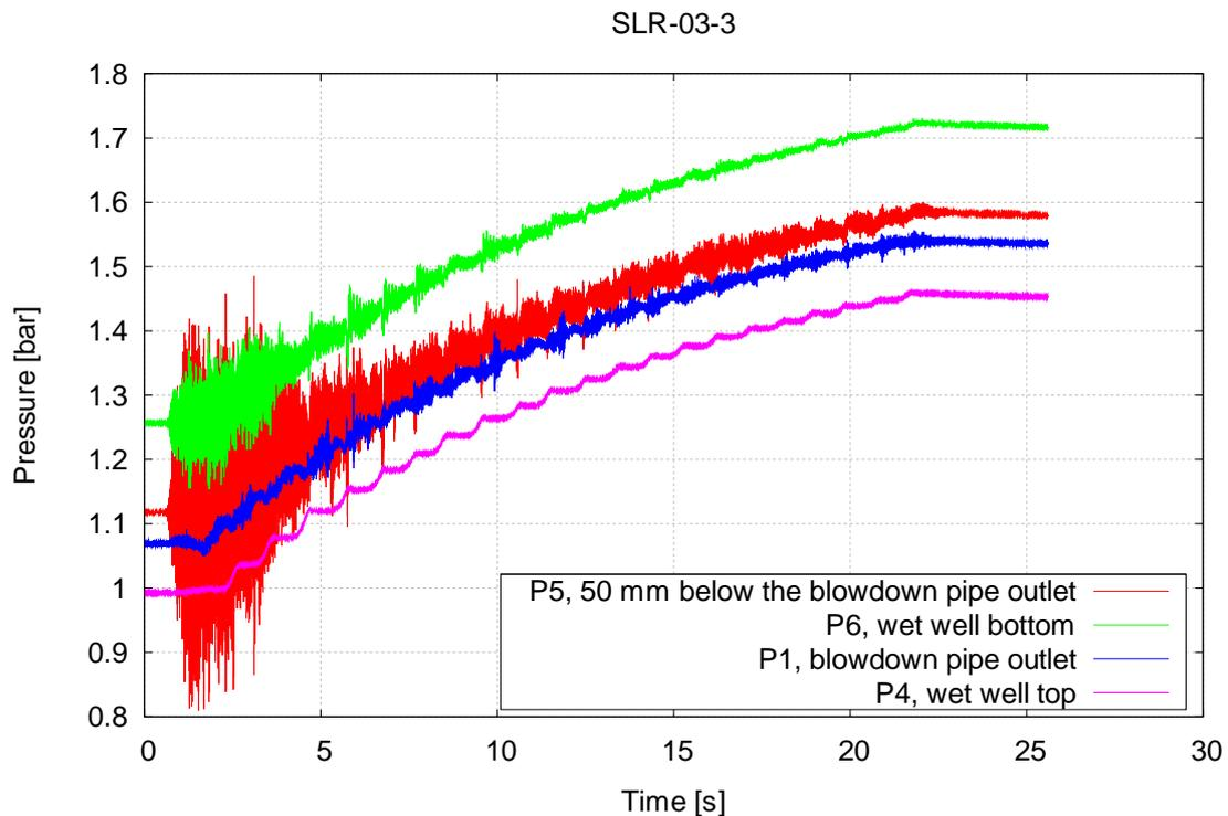
Figure 8. Pressures in the wet well in SLR-03-3.
