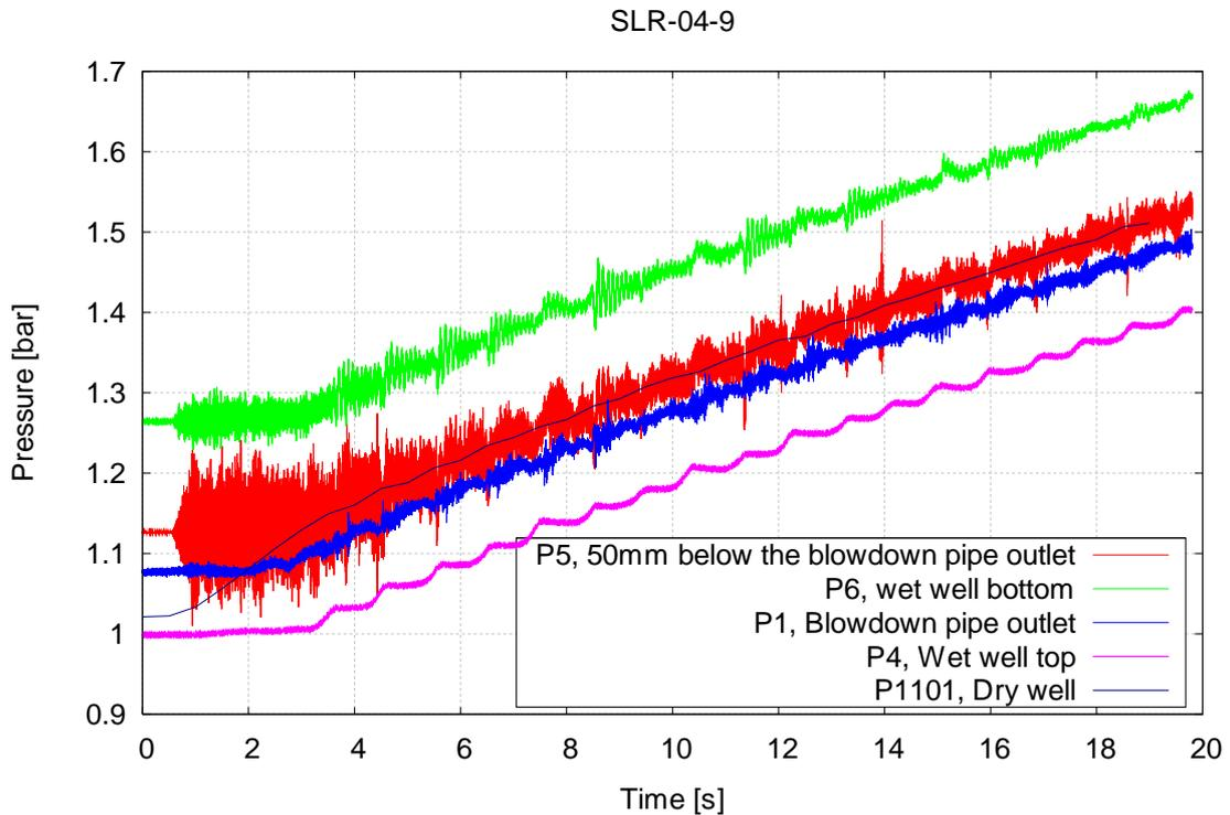
Figure 12. Pressures in the dry and wet well in SLR-04-9.
