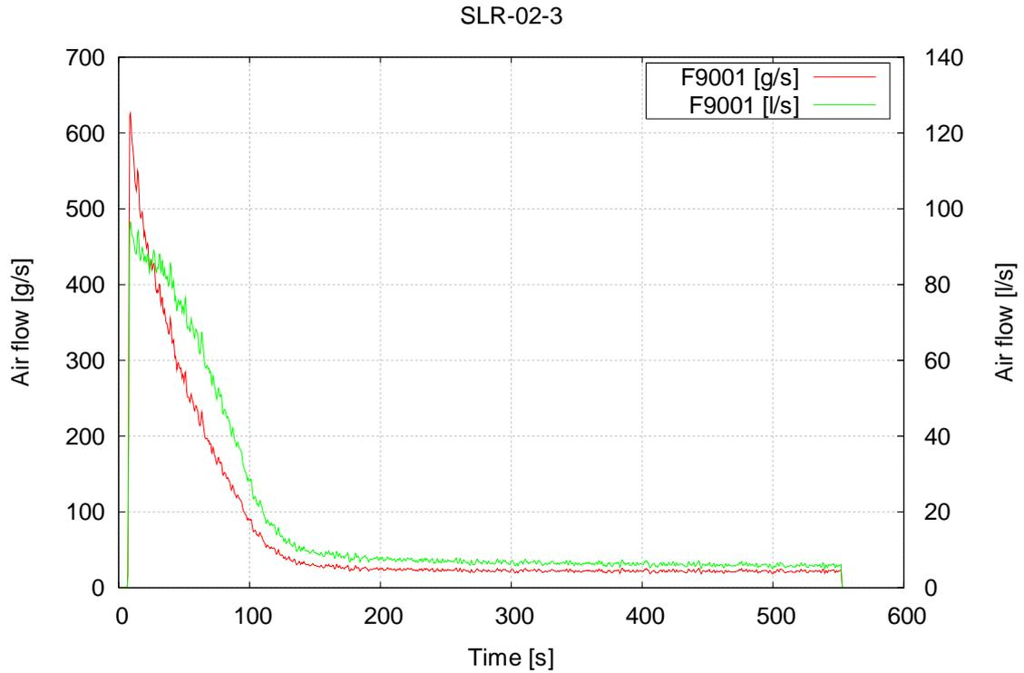
Figure 4. Volumetric and mass flow rate of air in SLR-02-3.
