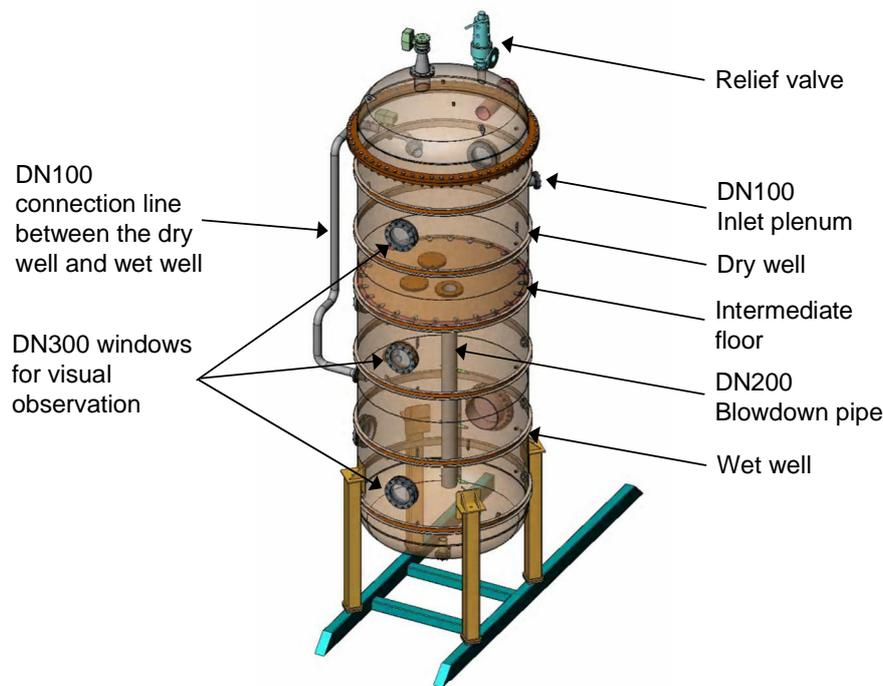
Figure 2. PPOOLEX test vessel.
