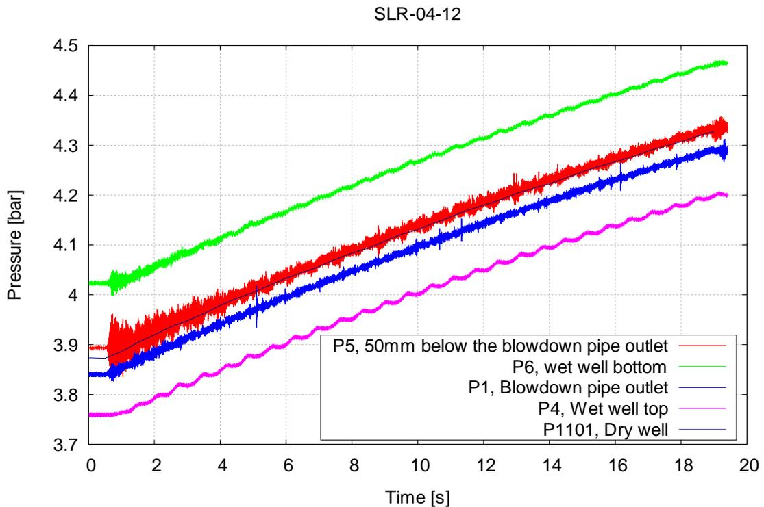
Figure 13. Pressures in the dry and wet well in SLR-04-12.
