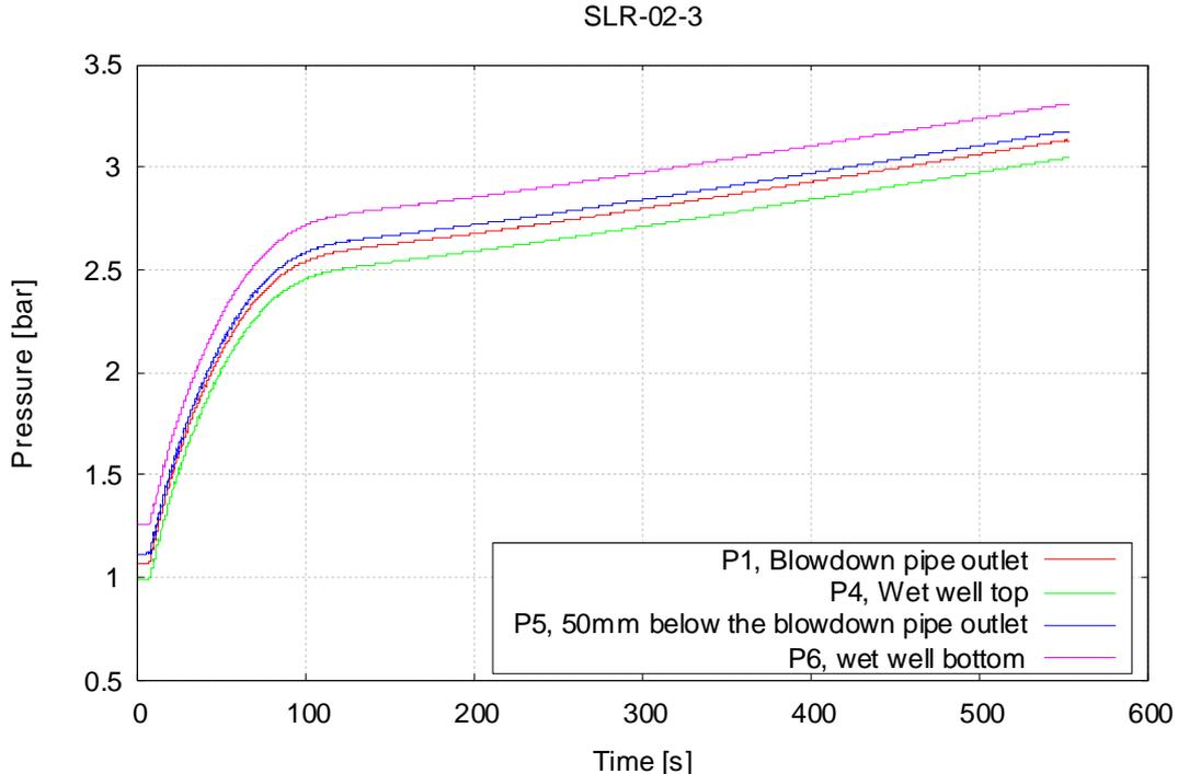
Figure 5. Pressure build-up in the wet well compartment in SLR-02-3.
