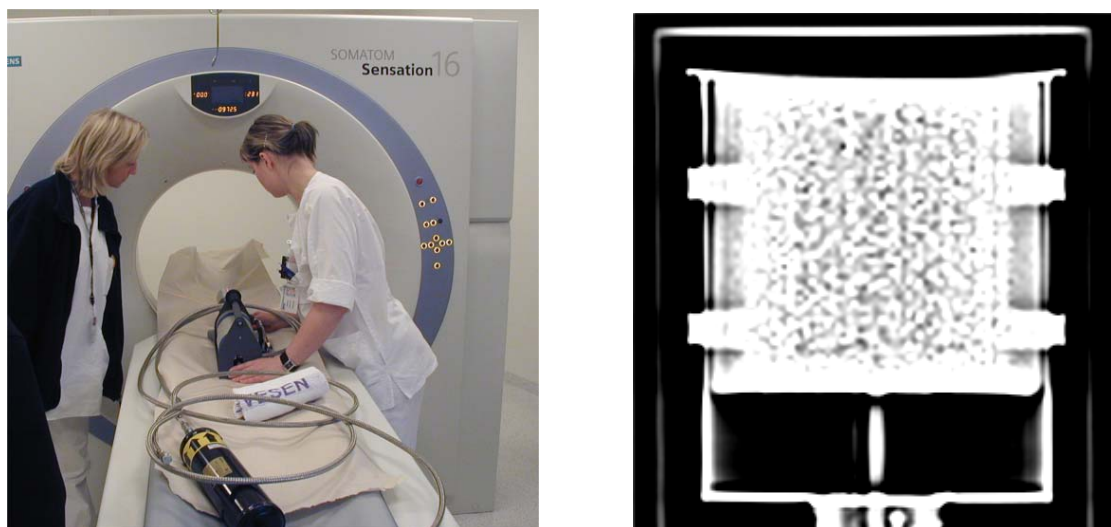
Figure 1. CAT scanning of the chosen detector for further characterizing and one view of the resulting scan.
