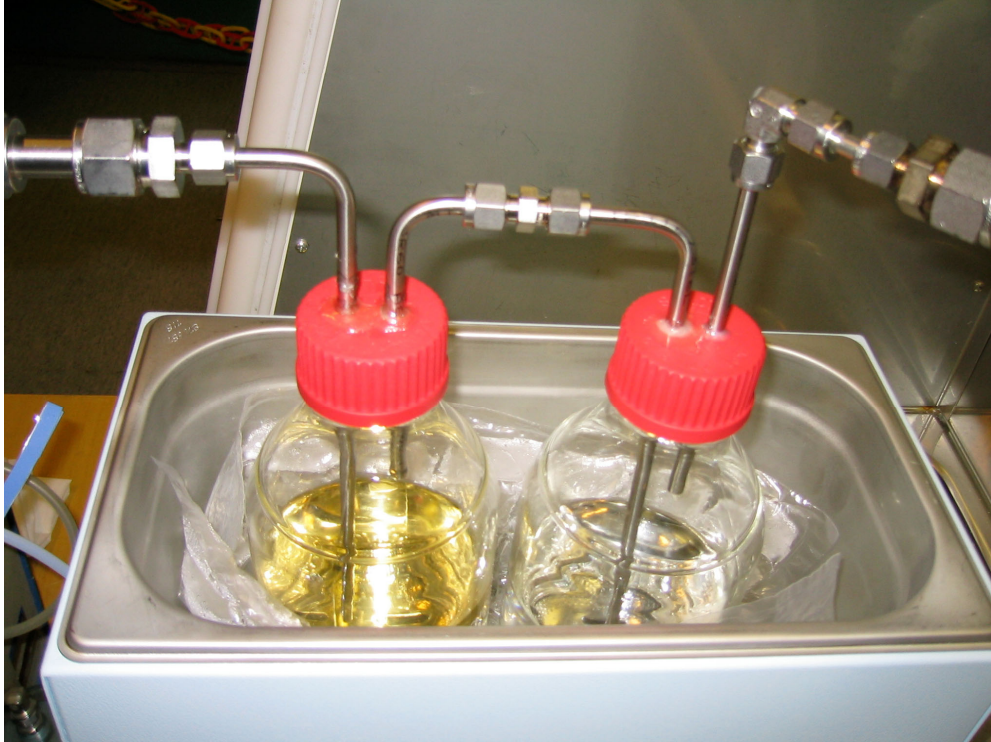
Figure 7: Two trapping bottles are shown. The solution in the first bottle has turned yellow when ruthenium has been trapped, whereas the solution in the second bottle is still uncoloured.
