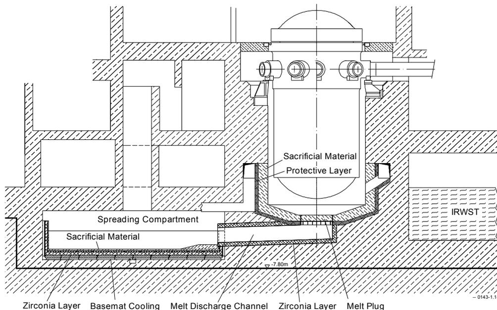
Figure 13 EPR Core Catcher.
