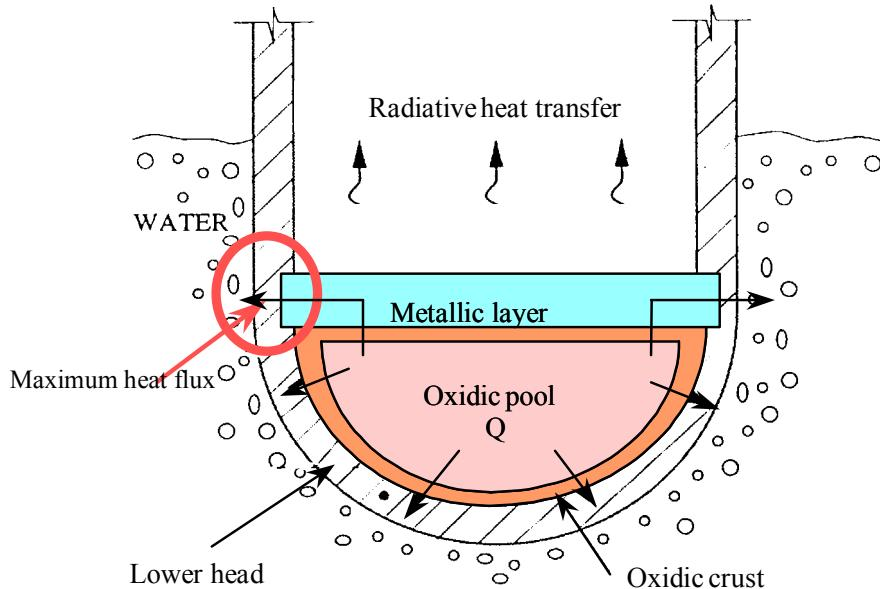
Figure 9 In-vessel Melt Retention.
