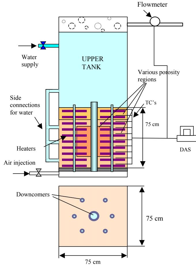
Figure 17 The Proposed POMEKO-GRAND Test Facility at KTH
