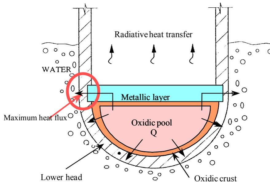
Figure 9 In-vessel Melt Retention.
