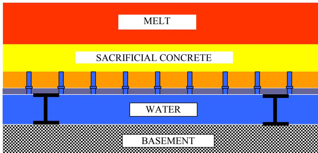
Figure 7 COMET: Bottom Water Injection through Plastic Tubes embedded in Sacrificial Concrete.
