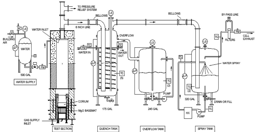
Figure 6 Basic Elements of the MET Apparatus.
