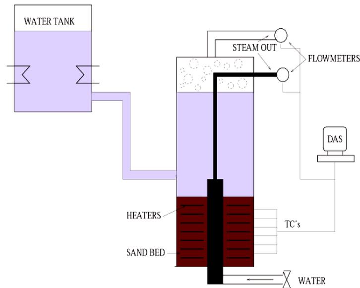
Figure 16 The POMECO Test Facility at KTH
