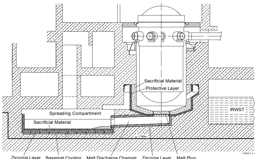
Figure 13 EPR Core Catcher.
