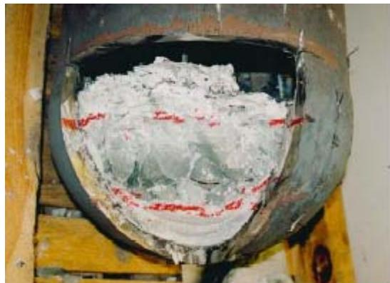
Figure 4 Post-test View of Solidified Melt for EC-FOREVER-5 Experiment.
