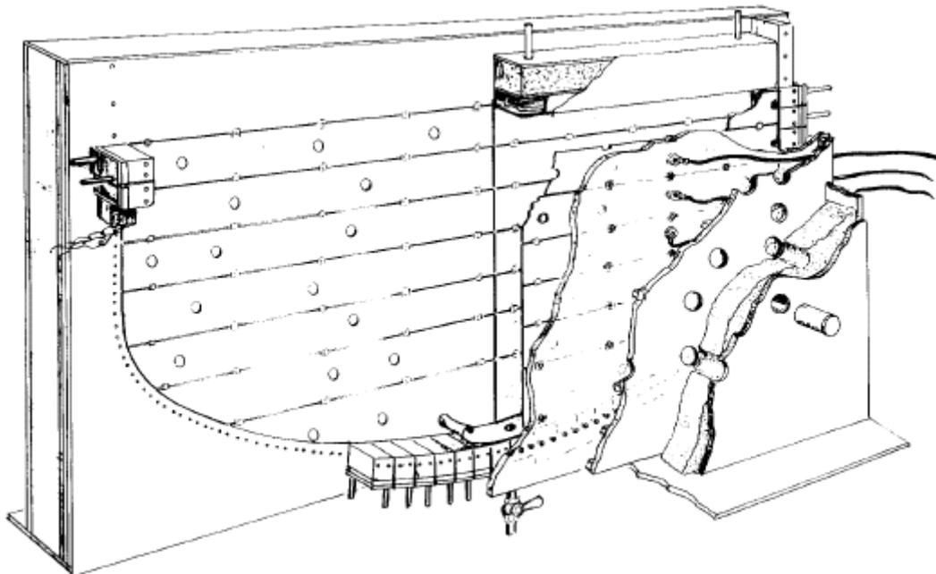
Figure 10 The COPO-I Facility at IVO in Finland (From Kymäläinen, et al., 1997)
