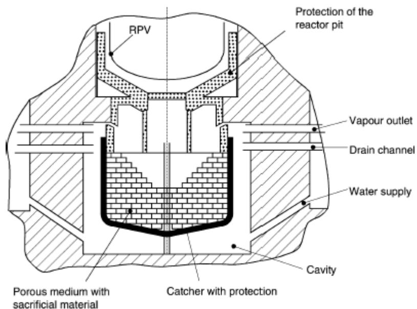
Figure 14 Tian Wan Core Catcher (From Seiler, J. M., 2003).
