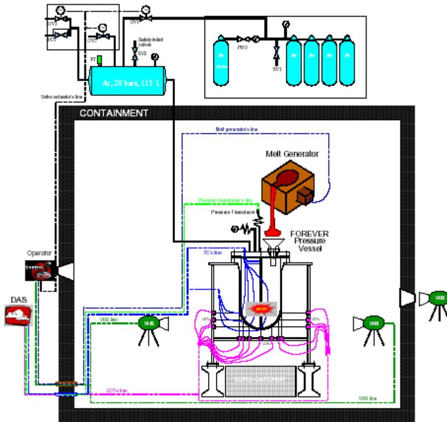
Figure 21 The FOREVER Test Facility at KTH
