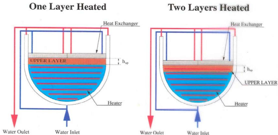
Figure 12 The SIMECO Test Facility at KTH.
