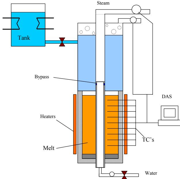
Figure 15 The COMECO Test Facility at KTH
