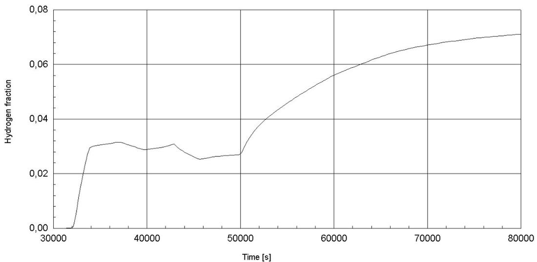
**Figure 10. Mole fraction of hydrogen when containment spray is started at  $t=50000$  s (sequence: S1H1-mod)**
