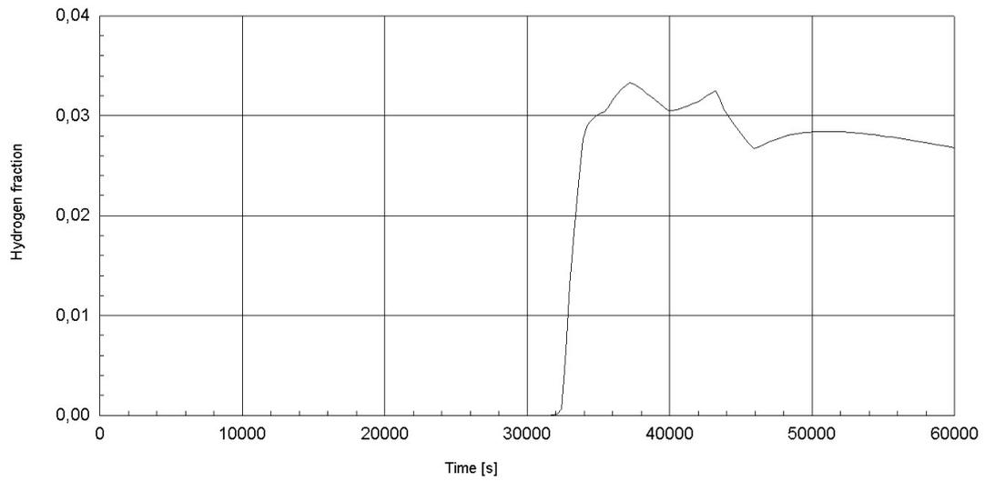
**Figure 7. Mole fraction of hydrogen in containment (sequence: S1H1)**
