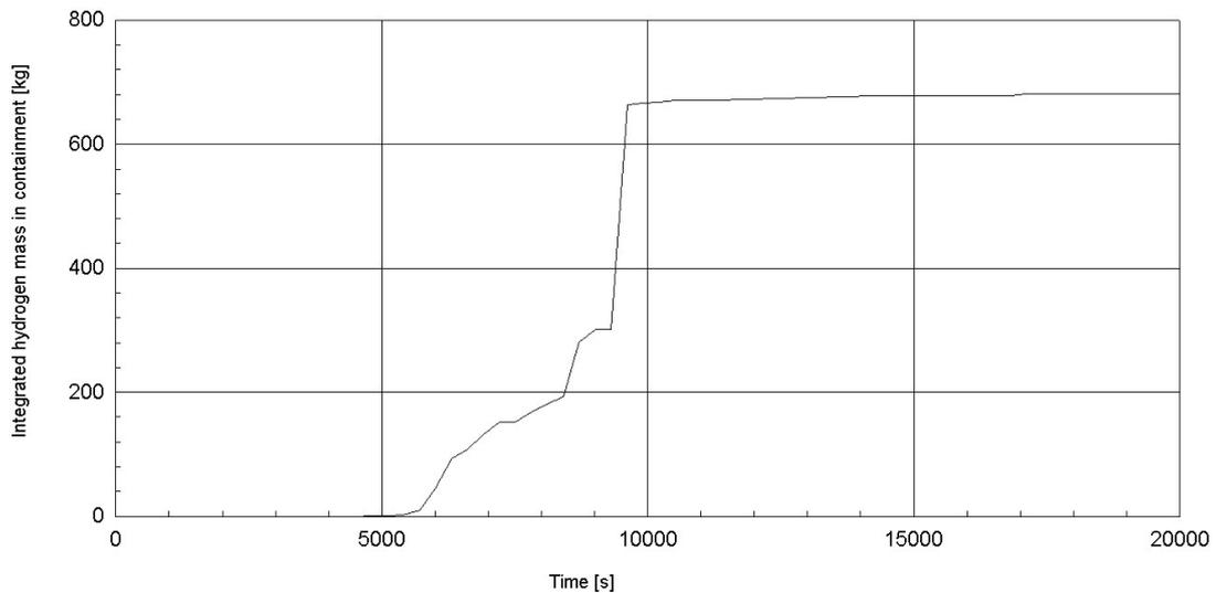
**Figure 14. Integrated mass in containment, sum of all hydrogen production phenomenon (sequence: T3LX4)**
