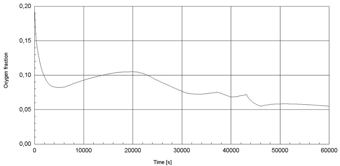
**Figure 8. Mole fraction of oxygen in containment (sequence: S1H1)**
