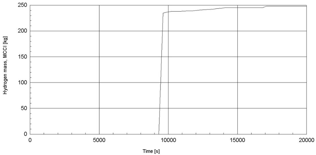
**Figure 16. Integrated mass of hydrogen from the MCCI (sequence: T3LX4)**
