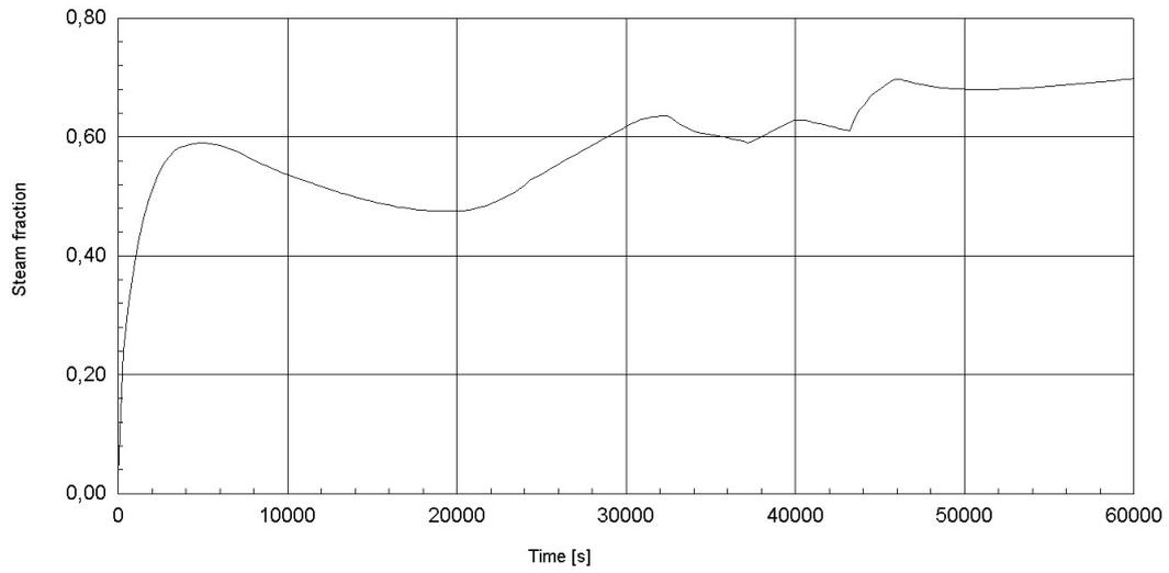
**Figure 6. Mole fraction of steam in containment (sequence: S1H1)**
