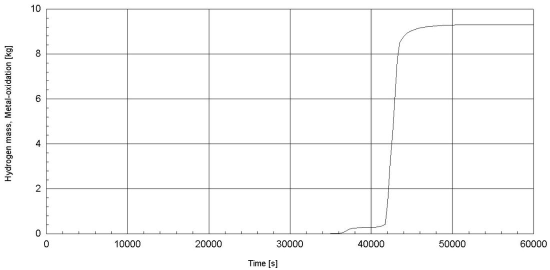
**Figure 4. Integrated mass of hydrogen from the metal (surfaces) oxidation (sequence: S1H1)**
