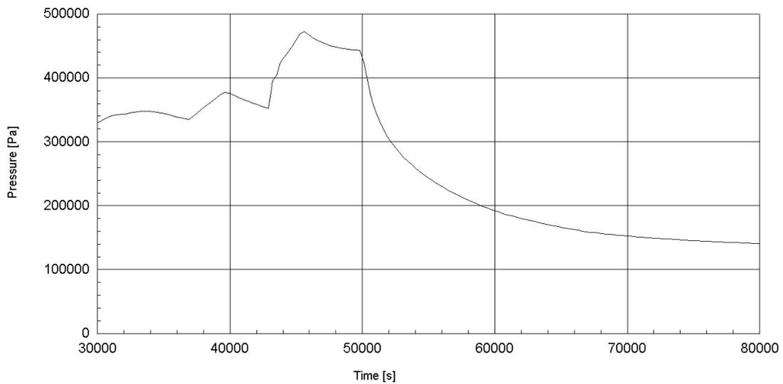
**Figure 12. Pressure in containment when spray is enabled at  $t=50000$  s (sequence: S1H1-mod)**
