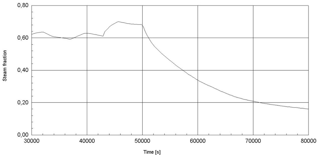
**Figure 9. Mole fraction of steam when containment spray is started at  $t=50000$  s (sequence: S1H1-mod)**
