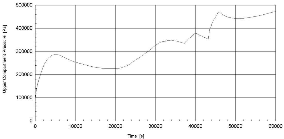
**Figure 1. Containment pressure (node: Upper compartment) as a function of time (sequence: S1H1)**
