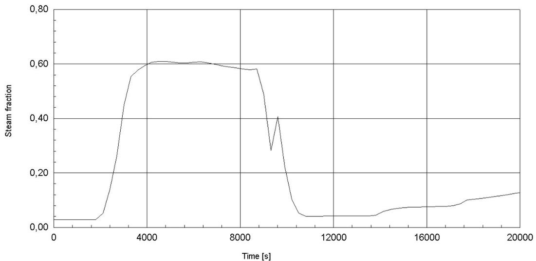
**Figure 17. Mole fraction of steam in containment (sequence: T3LX4)**
