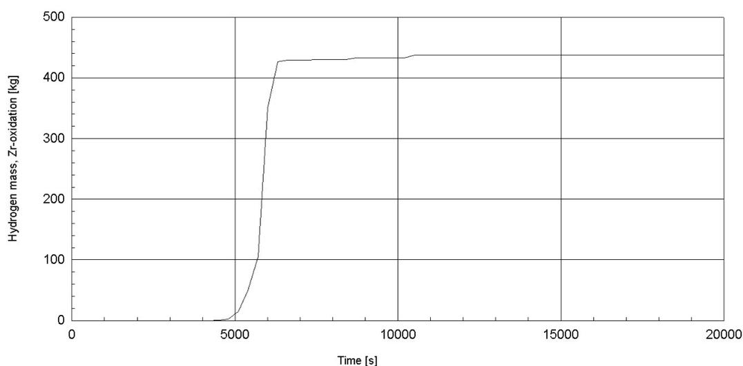
**Figure 15. Integrated mass of hydrogen from the Zirconium oxidation (sequence: T3LX4)**
