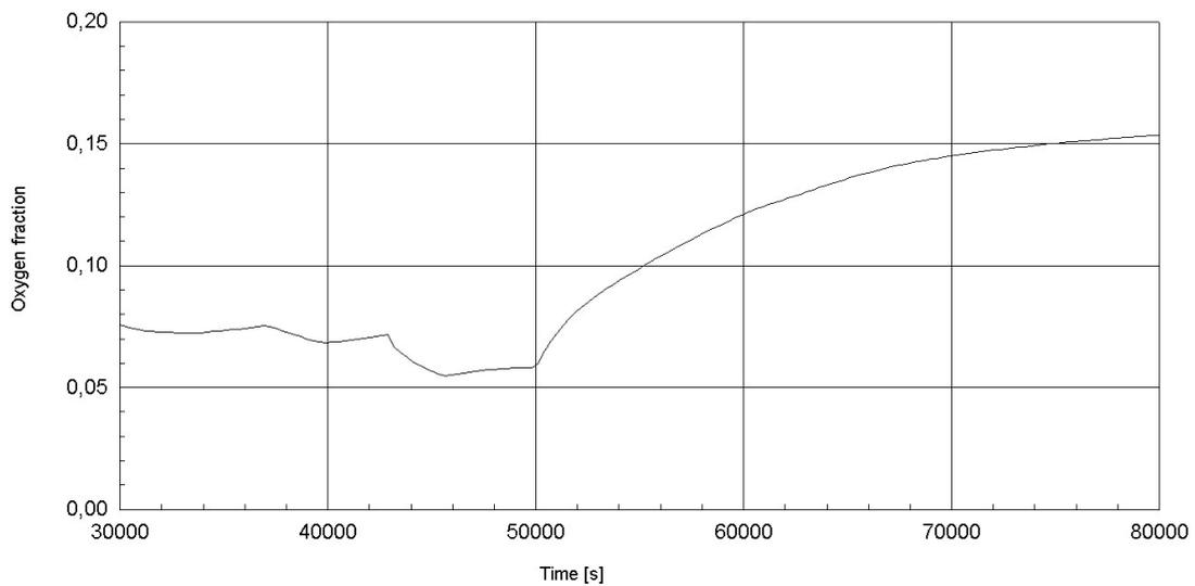
**Figure 11. Mole fraction of oxygen when containment spray is started at  $t=50000$  s (sequence: S1H1-mod)**
