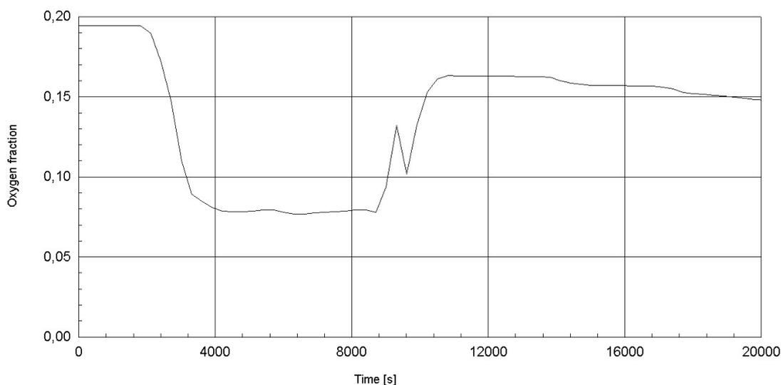
**Figure 19. Mole fraction of oxygen in containment (sequence: T3LX4)**
