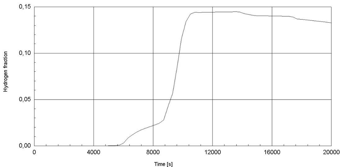
**Figure 18. Mole fraction of hydrogen in containment (sequence: T3LX4)**
