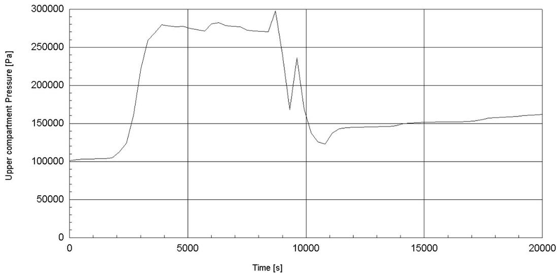
**Figure 13. Containment pressure (node: upper compartment) as function of time (sequence: T3LX4)**
