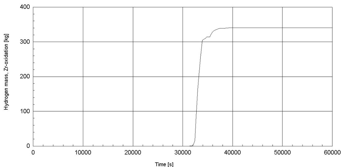
**Figure 3. Integrated mass of hydrogen from the Zirconium oxidation (sequence: S1H1)**
