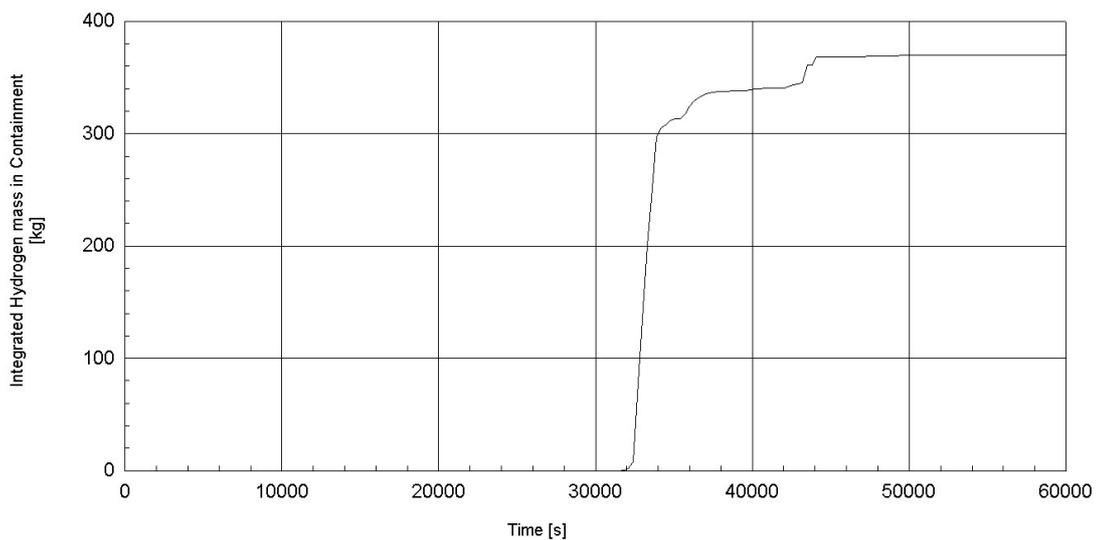
**Figure 2. Integrated mass in the Containment. Sum of all hydrogen production phenomena (sequence: S1H1).**
