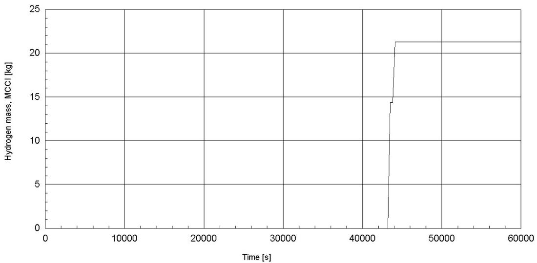
**Figure 5. Integrated mass of hydrogen from the MCCI (sequence: S1H1)**
