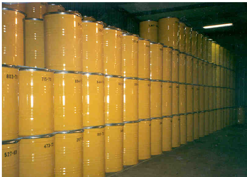
Figure 7. Reconditioned old drums with low-level solid radioactive waste in an unheated storage building at Studsvik.
