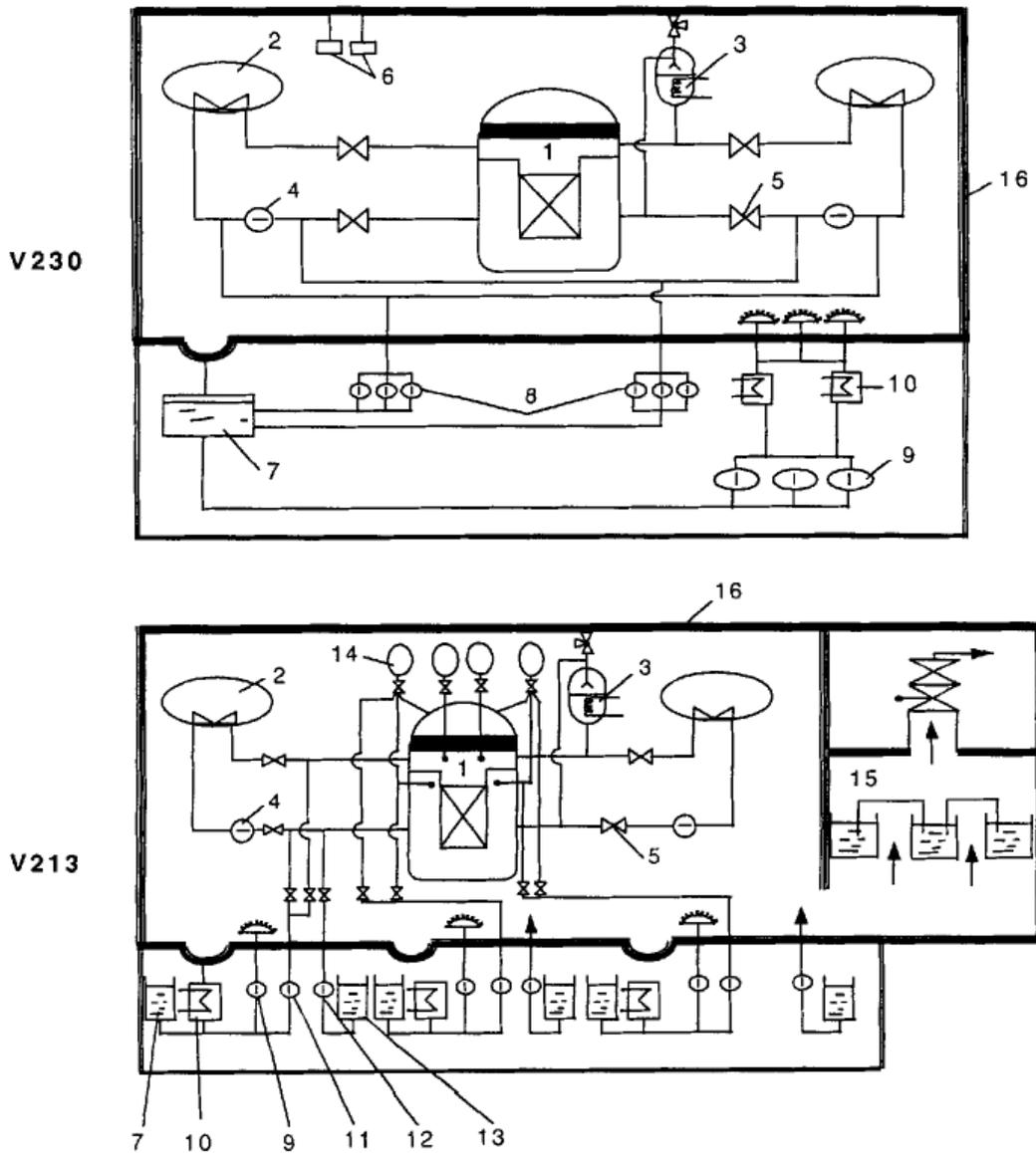
Fig. 3.2. Differences between VVER-440 reactor designs 230 and 213 (Source: Ref. 1)
