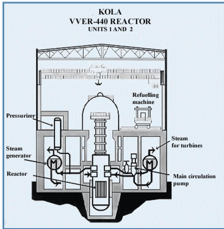
Fig. 3.1. The reactor building of a VVER-440/230 reactor (Kola NPP units 1 and 2).
