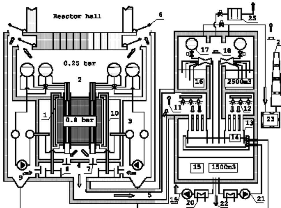
Fig. 2.3. Accident "localization system" of an RBMK reactor (Source: Ref. 1)
