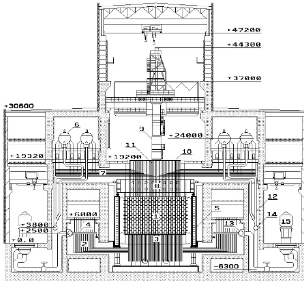
Fig. 2.8. Cross-sectional view of units 1 and 2 of Leningrad NPP (Source: Ref.1)
