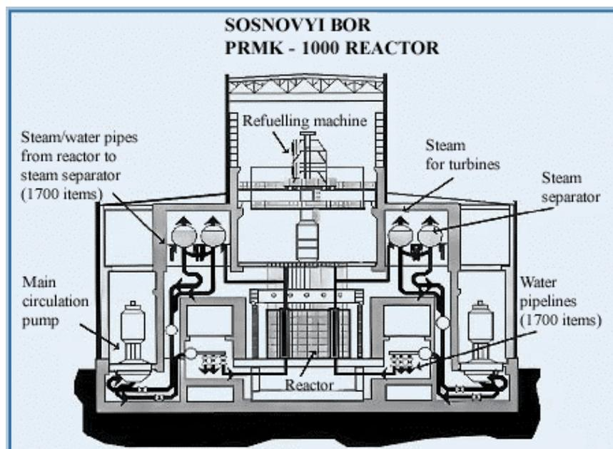
Fig. 2.1. The reactor building of an RBMK-1000 reactor (Leningrad nuclear power plant) (Source: [www.stuk.fi/english/npp](http://www.stuk.fi/english/npp))
