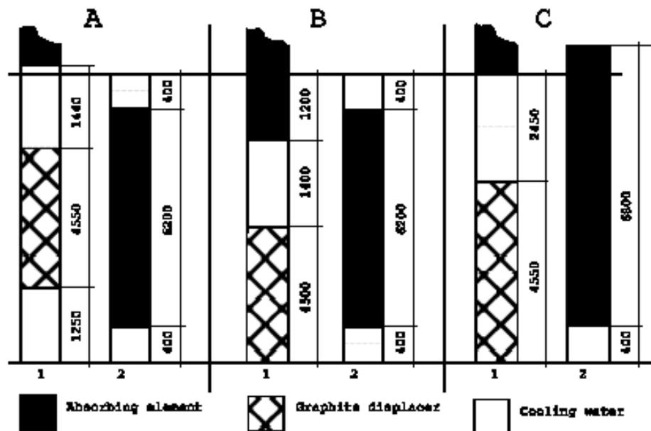
Fig. 2.2. Control rod positions at different levels in the core (Source: Ref. 1)
