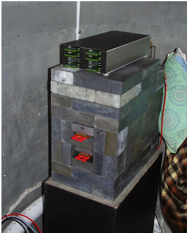
Figure 2. Low-level Geiger-Müller multi-counter system at Risø National Laboratory. The picture shows two multi counters, one on top of the other, in a 10-cm lead shield.
