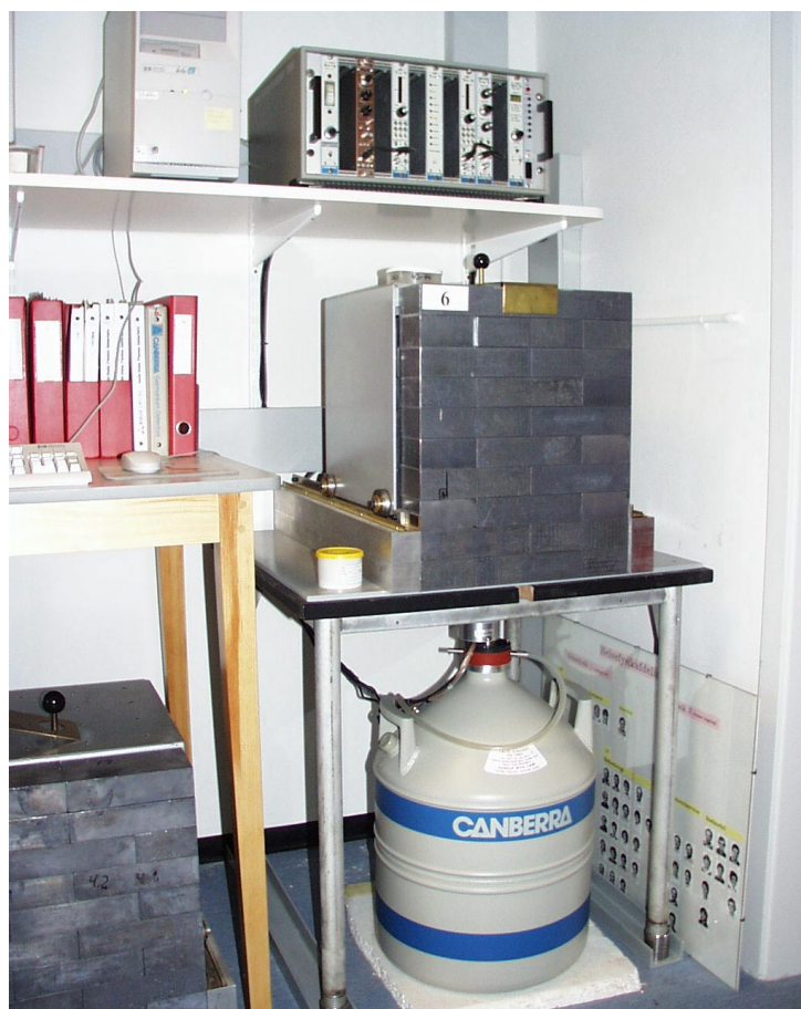
Figure 1. Low-level HPGe spectrometer system at Risø National Laboratory. The samples are placed in the lead shield on the table.
