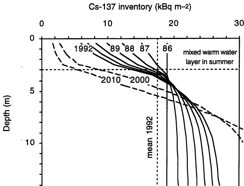
Fig.: Chernobyl Cs-137 in a Swedish lake: Observed, estimated and projected values of mean sediment inventories at different depths during the years after the nuclear fallout in 1986.
