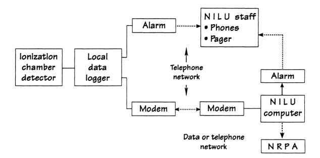
B) Block diagram of the Norwegian gamma spectrometric stations and alarm response
