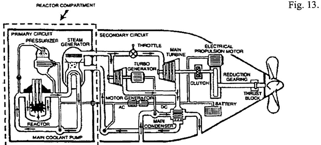
Figure 13. Layout of a dispersed PWR nuclear propulsion plant.
