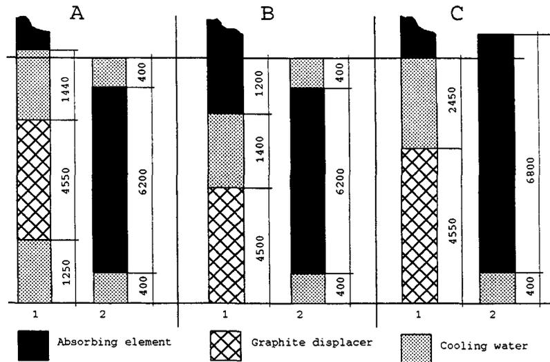
Figure 11. Control rod positions at different levels in the core
