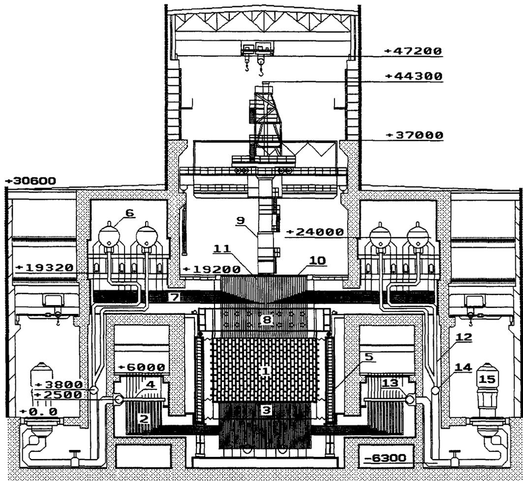
Figure 9. Cross-sectional view of unit 1 and 2 of the Leningrad NPP
