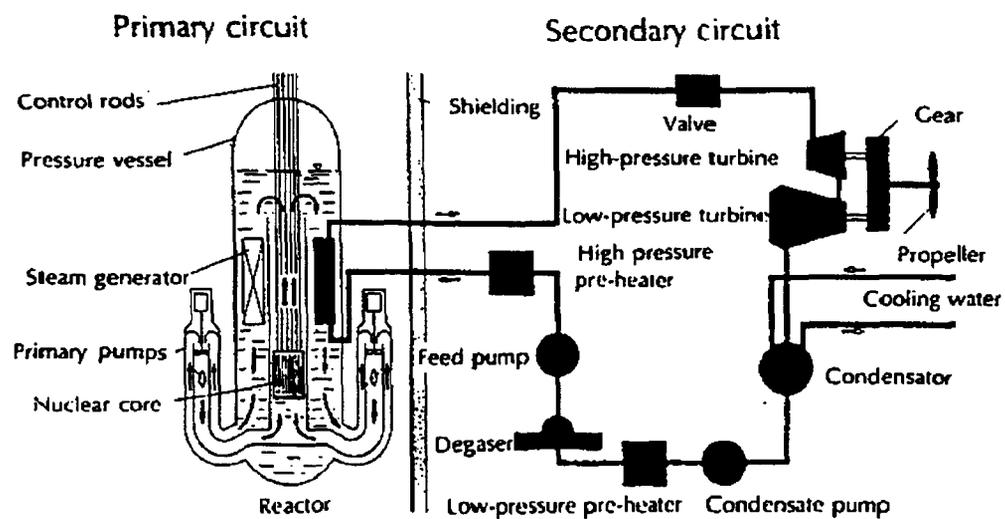
Figure 14. Layout of an integrated nuclear propulsion plant
