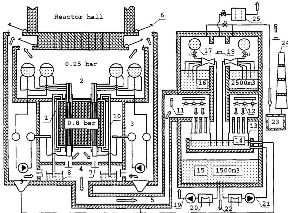
Figure 12. Accident localization system of RBMK reactor
