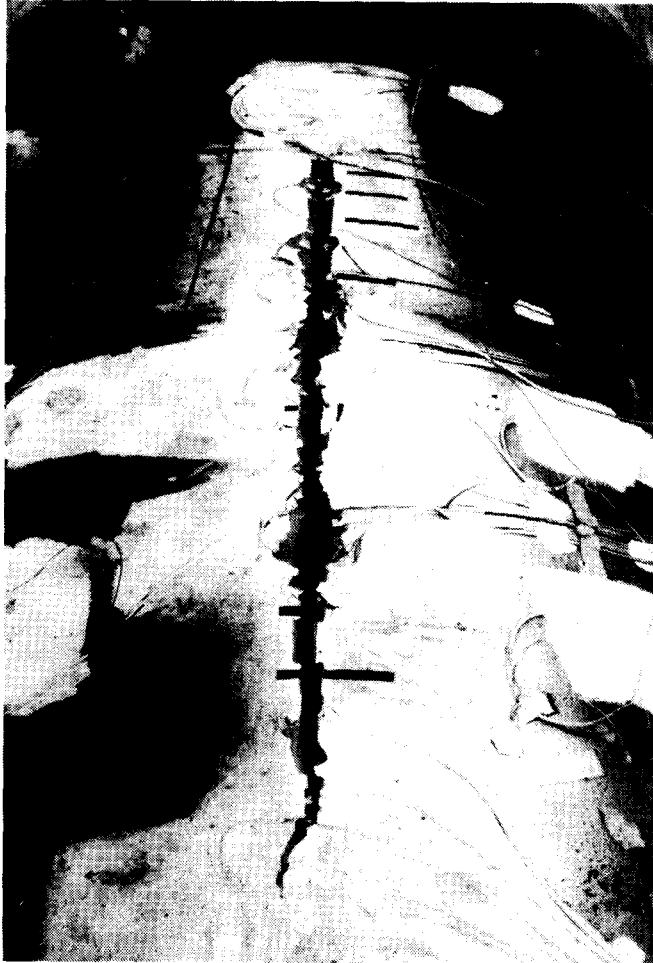
Fig. 18. An overview of the leak region in the HC2-pressure vessel test [20].
