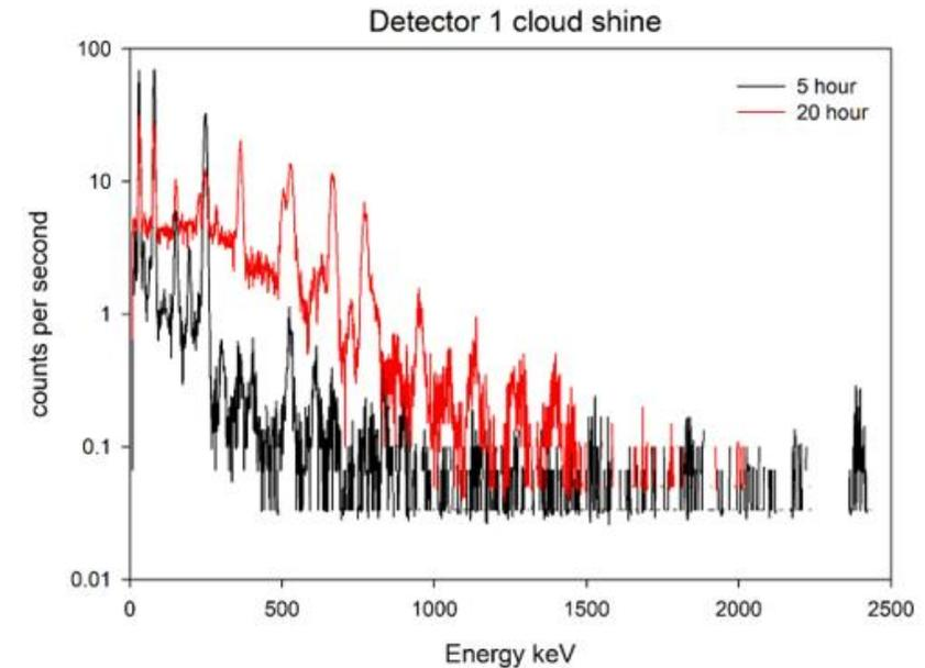
5 hour and 20 hour cloud shine spectra for Detector 1.
