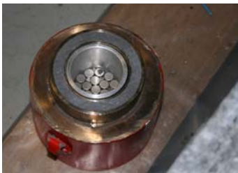
Magnets in the bottom of the shielding for the sample flask, to prevent chips to pack up in the filter.
