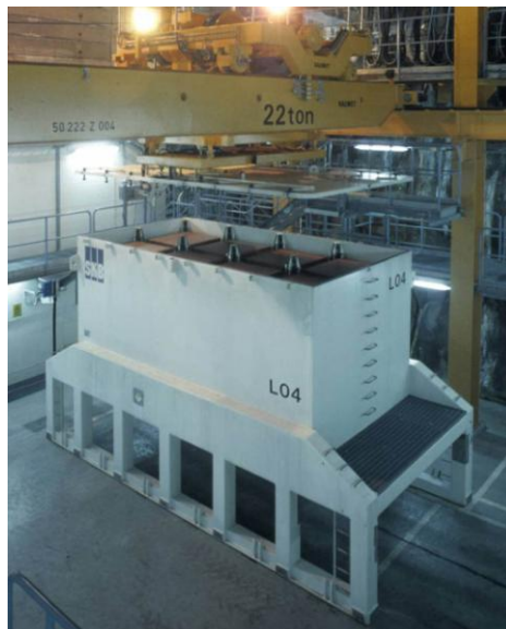
Figure 2: SKB shielded transport container.
