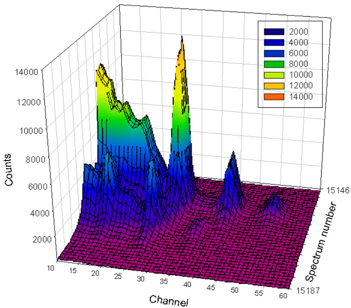
Figure 13. Graphical representation of the transition between Source 3 ( $^{192}\text{Ir}$ ) and Source 4 ( $^{75}\text{Se}$ ).
