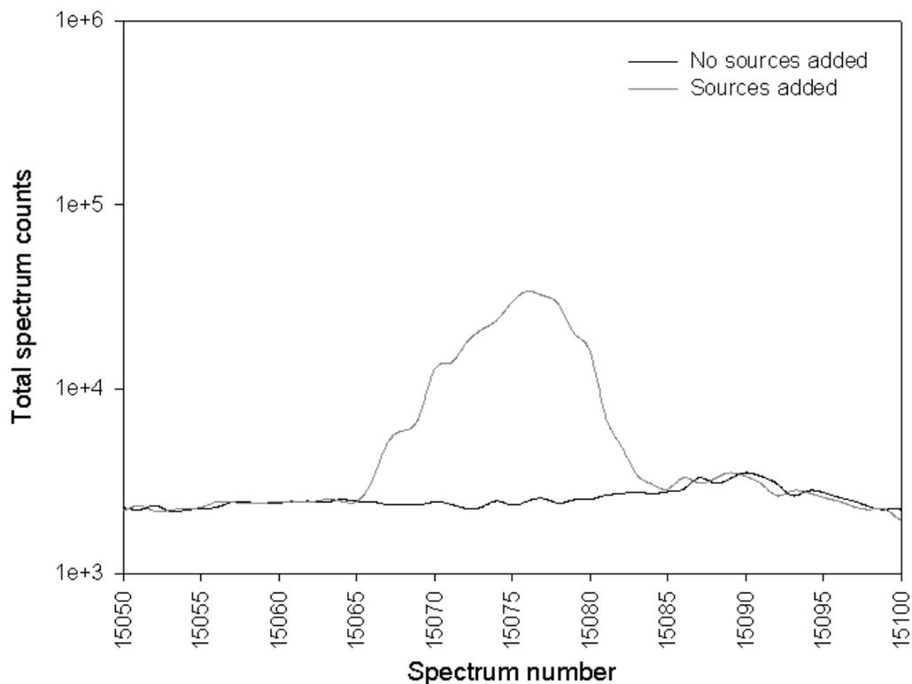
Figure 7. Total spectrum counts over the part of Trip 2 for which Source 1 was visible.
