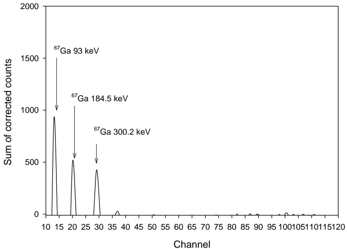
Figure 16. Sum of background corrected counts for spectra between 15232 and 15246 for Source 4.
