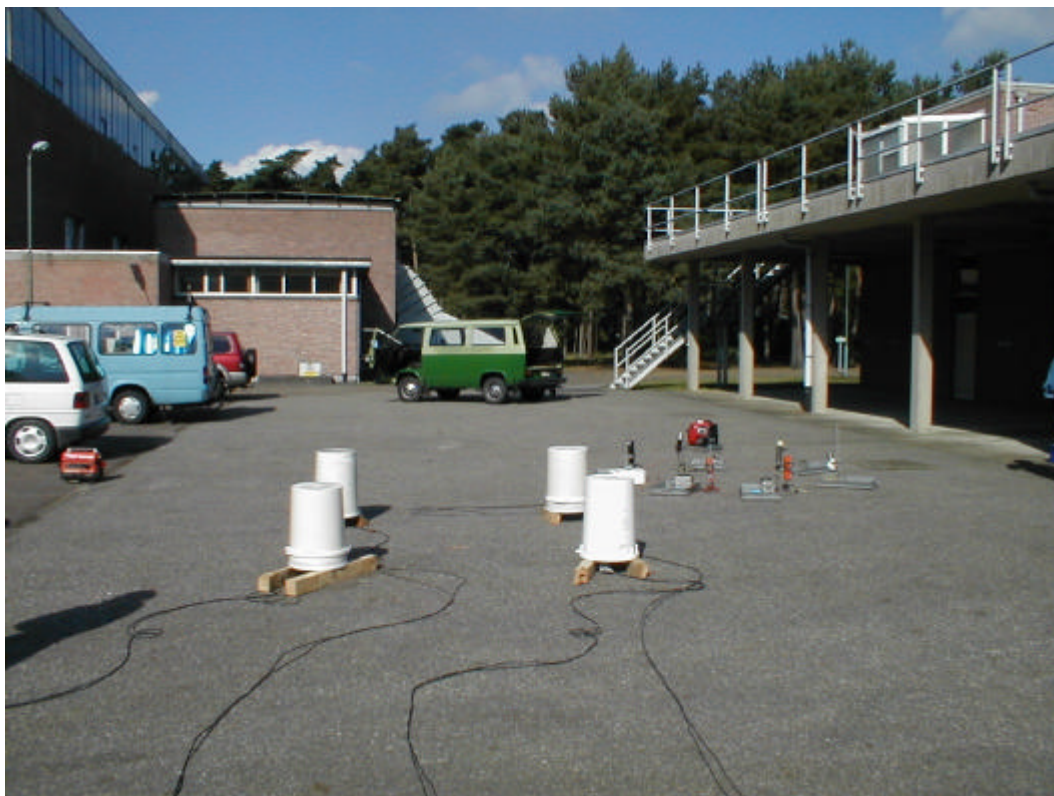
Figure 16. NaI detector calibration. The white barrels in the foreground contain the DK-NaI detectors (setup 1).
