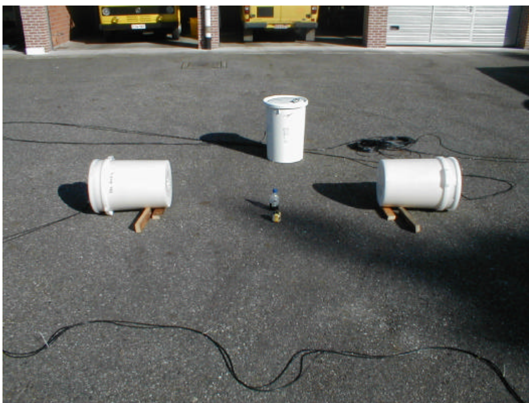
Figure 17. NaI detector calibration. Setup 2.
