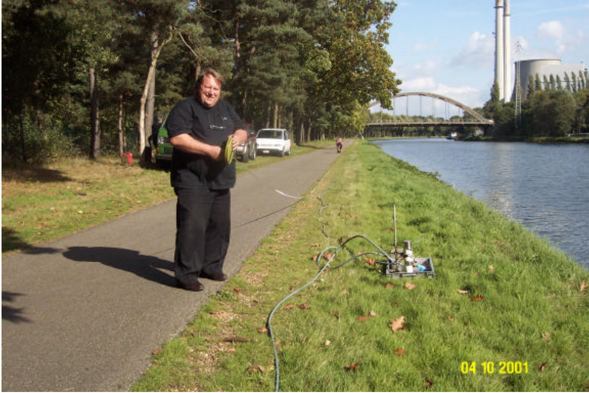
Figure 15. Setting up NaI detectors along the channel. Lidar scanning was performed the same place on Friday, October 5 th .
