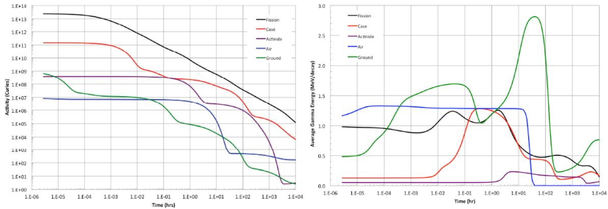
Figure 1. Radiation source term for the Hiroshima detonation (aggregate decay of ~1200 radionuclides) (left) and average total gamma energy released per decay for each source term (right). From: Spriggs G.D. and Egbert, S.D., LLNL-TR-814785, 2017)
