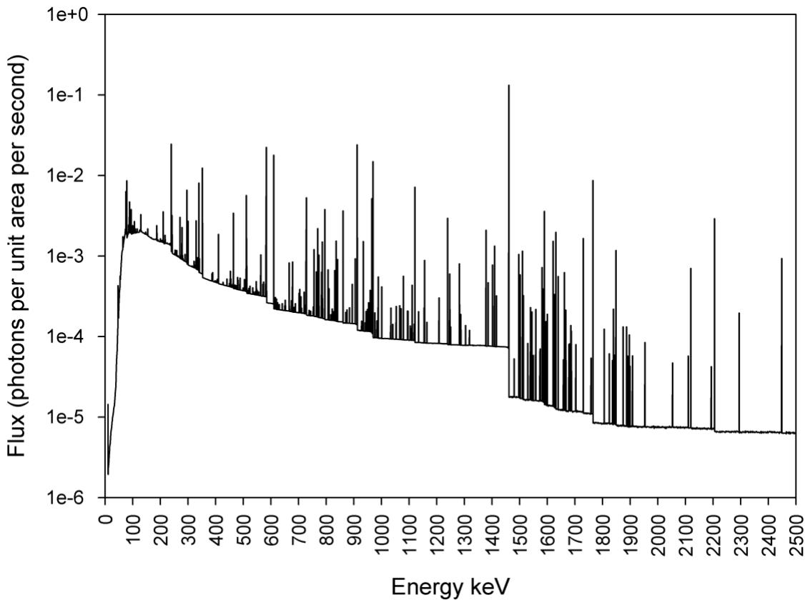
Figure 9. Background photon flux as added to the spectra.
