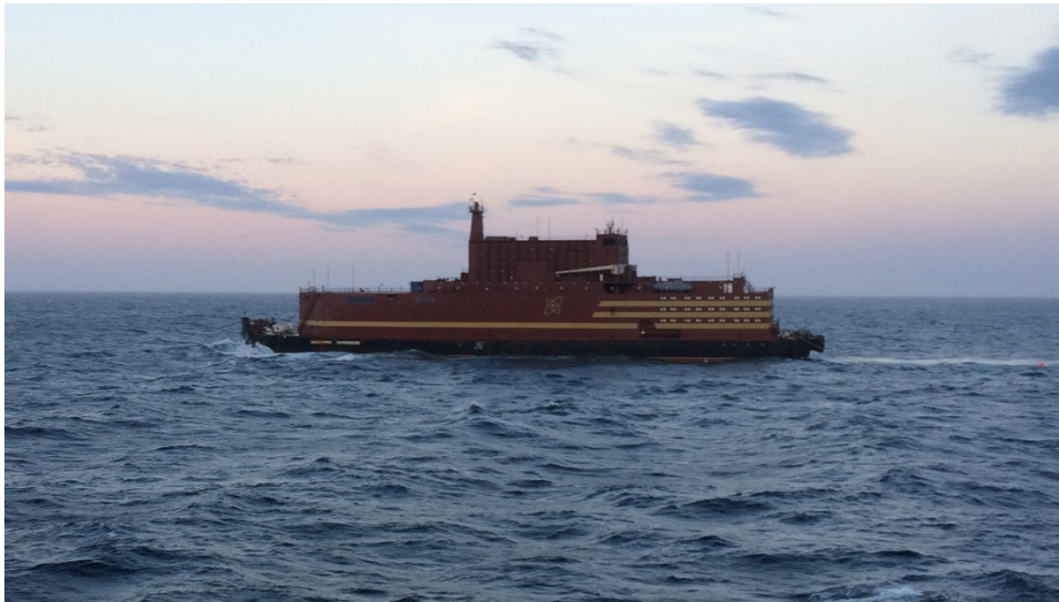
Figure 15: FNPP "Akademik Lomonosov" (2 x 150 MWt reactors) during towing from St. Petersburg to Murmansk in May 2018 (Photo: Øyvind Aas-Hansen).
